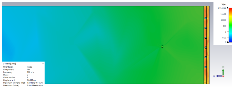
(b) Section view of the LoCMOS electrode with an E. coli cell present.
