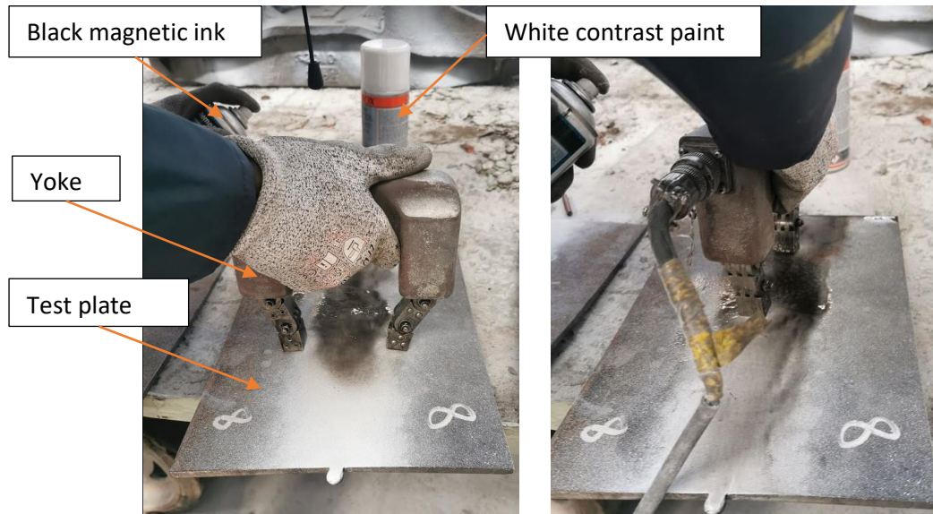
Figure 54: MT performed on the welded
