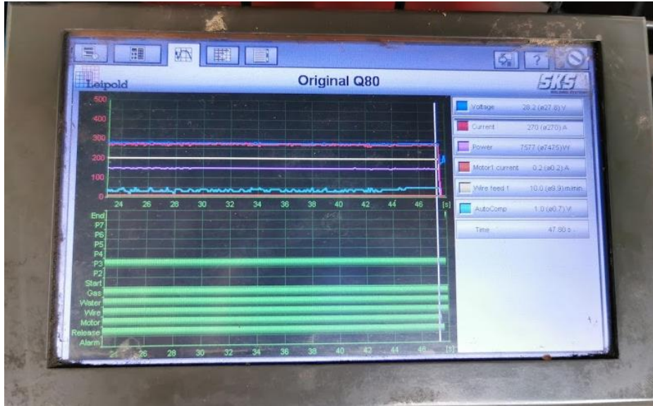
Figure 52: Welding parameters graphs for root run and capping run
