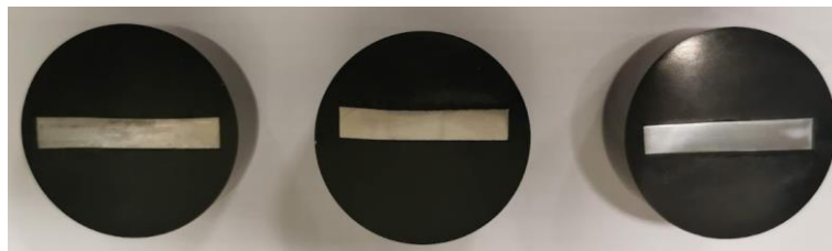
Figure 23: Mounted specimens for hardness test
