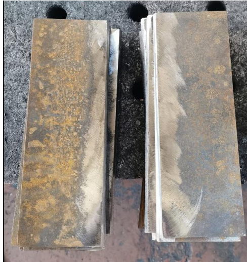
Figure 44: Waterjet cut steel plates
