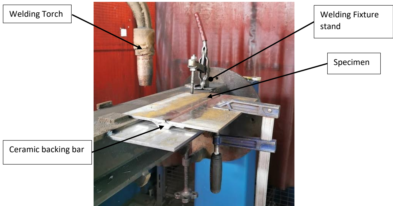
Figure 46: Fixture arrangement for fixing specimen
