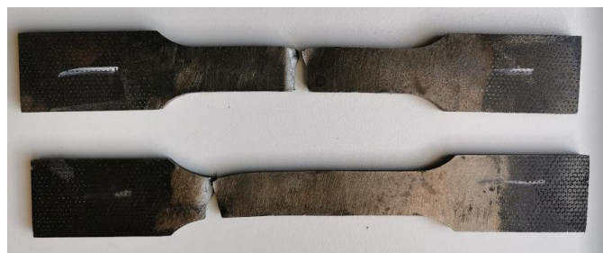
Figure 38: Fatigue tested specimen showing the location of fracture
