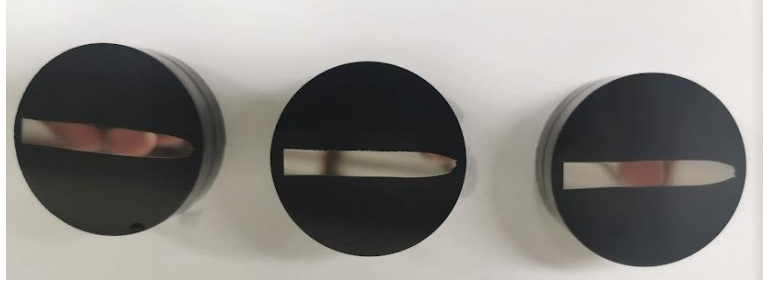
Figure 22: Mounted specimens for macrostructural examination
