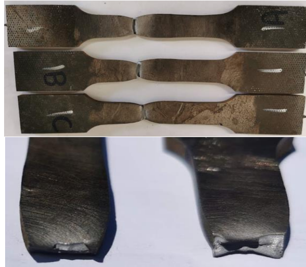
Figure 37: Shear bands mode of fracture for tensile test
