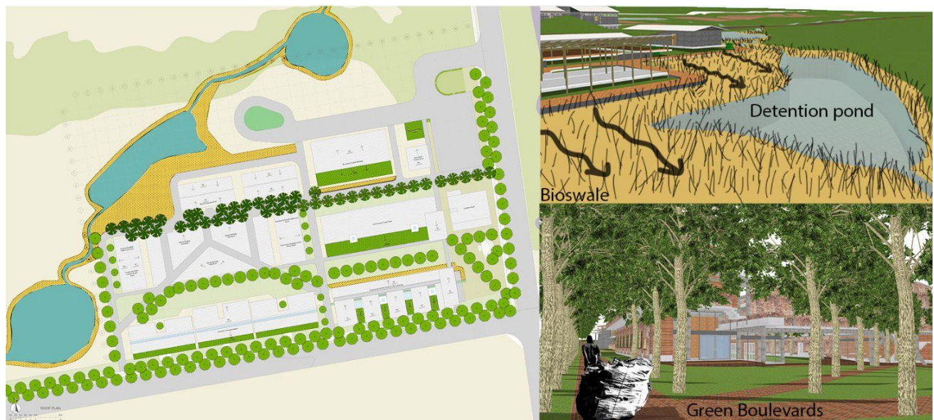
FIGURE 3.0 - The site strategies employed which consist of greenboulevards, bioswales and detention ponds (Author 2023)
