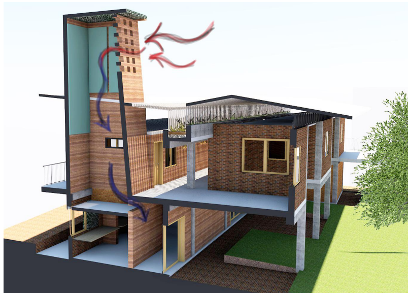
Figure 3.20 - A perspective section demonstrating ecological and passive design, with an evaporative cooling tower, wind scoop, double insulated roof, bioswale gutter for water harvesting and natural lighting into the rooms from the translucent sheeting allowing well lit interior spaces (Author 2022).
