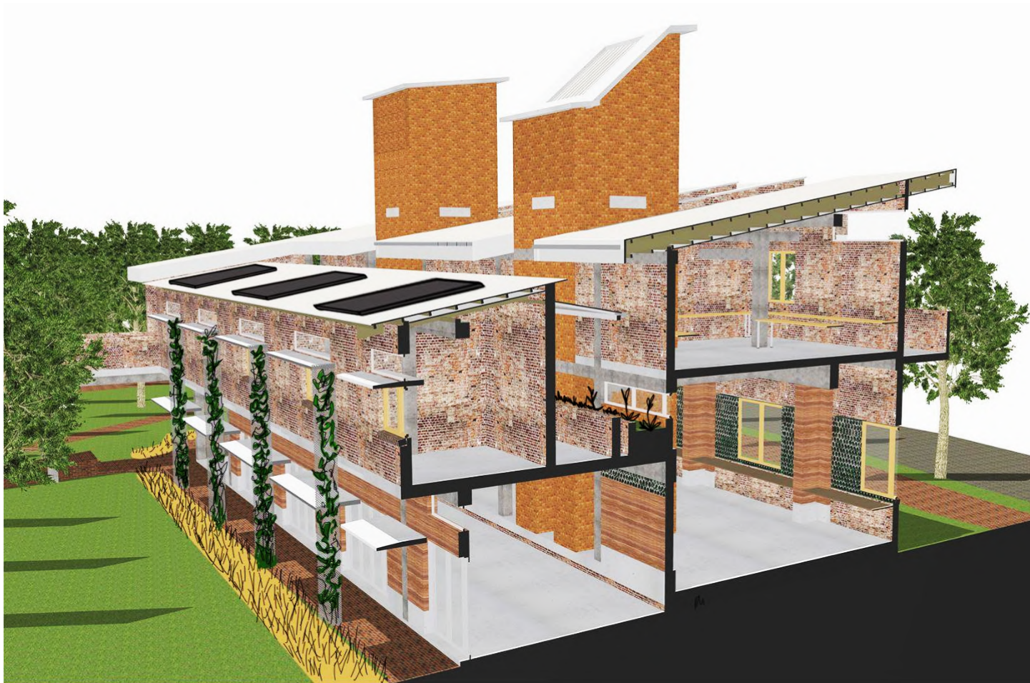
FIGURE 3.1 - The building strategies employed on site; green screens (shielding western light), photovoltaic panels, light shelves to the north, ambient lighting from southern clearstory windows and green roofs (extensive) (Author 2023)
