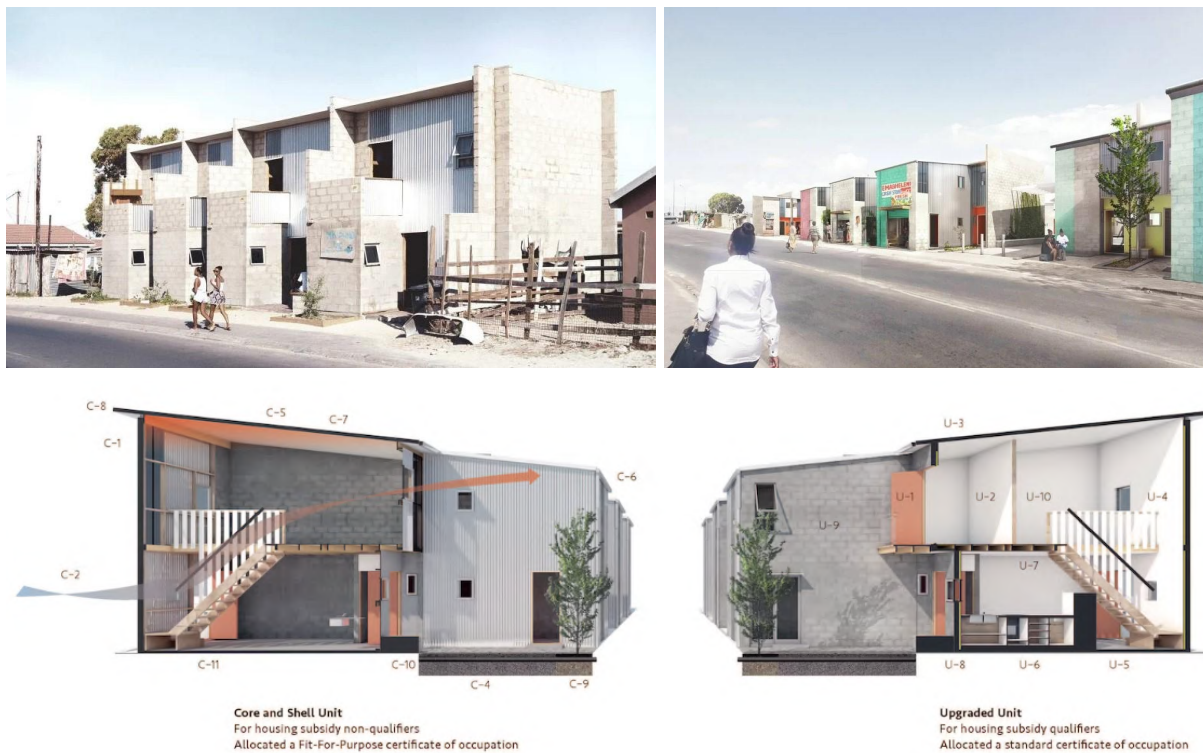
Figure 2.2 - Empower Shack showing the robust and simple design with future use renders (Above) (De zeen 2017) with a section to show the shell and how one may appropriate the space over time (Left to Right, Below) (Architizer 2020).
