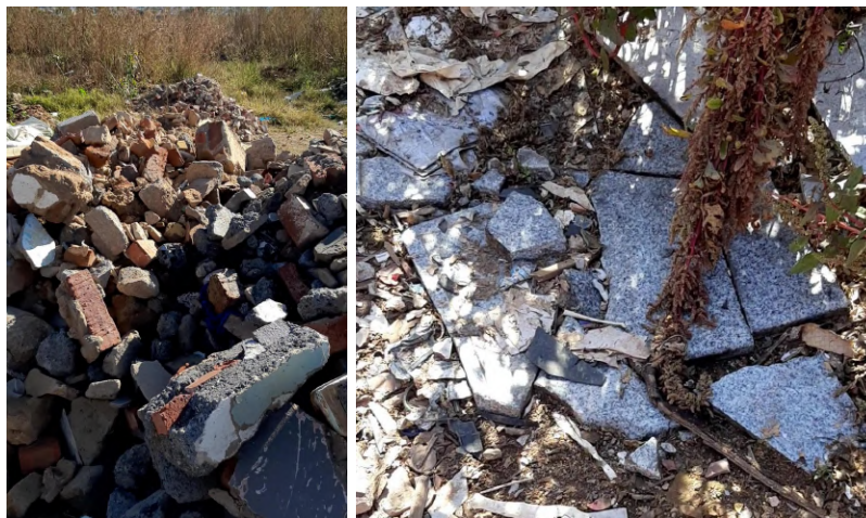
Figure 3.14 - Open Green Space Rubble dumping, of which there are mixed aggregates, bricks, stones, concrete blocks and sand as well as more valuable items such as broken tiles and Granite pieces (Right). These can be used for infill walls, or as aesthetic pavers and spaces in the project (Author 2022).
