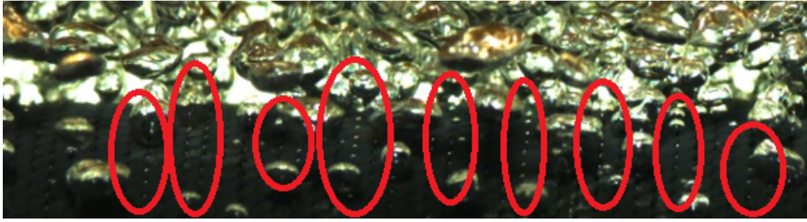
Figure 7.10: Vapour entrapment in the GEWA-B5 re-entrant cavities in pool boiling at 20\text{ kW/m}^2 and 5^\circ\text{C} in R134a
