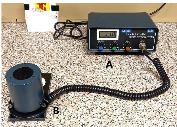
Figure S4 Diffusion System Ltd EEL model 43D Smoke Stain Reflectometer, where A is the control unit and B measuring head.
