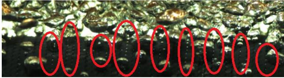
Figure 4-6. Bubble ejection impedance in coated GEWA-B5 re-entrant cavities in pool boiling at 20\text{kW/m}^2 and 5^\circ\text{C} in R134a
