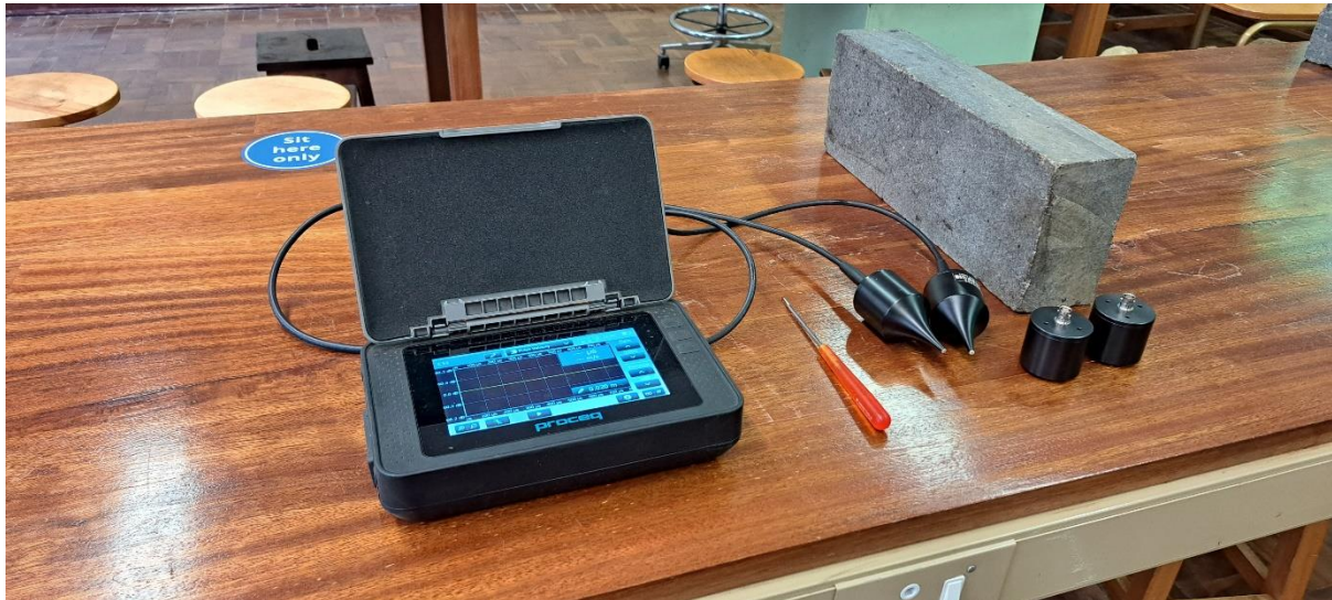
Figure 26. PUNDIT PL-200 ultrasonic pulse velocity apparatus with attached rough surface transducers, pictured next to a gabbro sample stone, alongside detached 54kHz standard transducers
