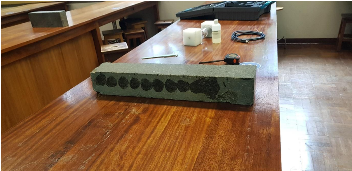
Figure 25. Gabbro sample block with stains from ultrasonic couplant. In the background is a bottle of ultrasonic couplant and the rough surface transducers in their polystyrene protective blocks
