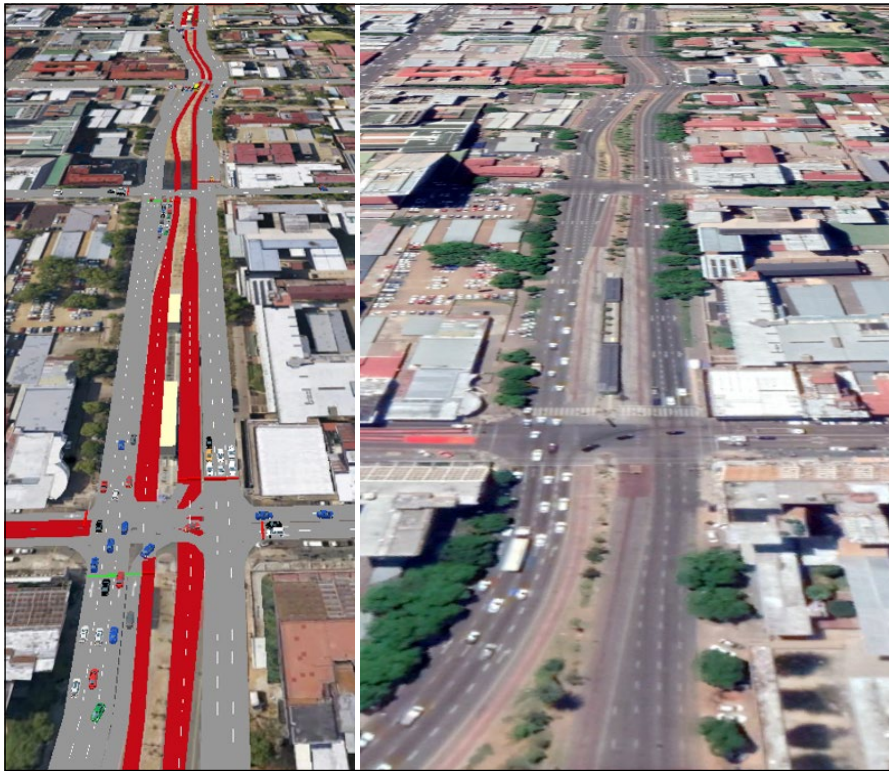
Figure 3 VISSIM model (left) of the Nana Sita BRT corridor (right), Tshwane
