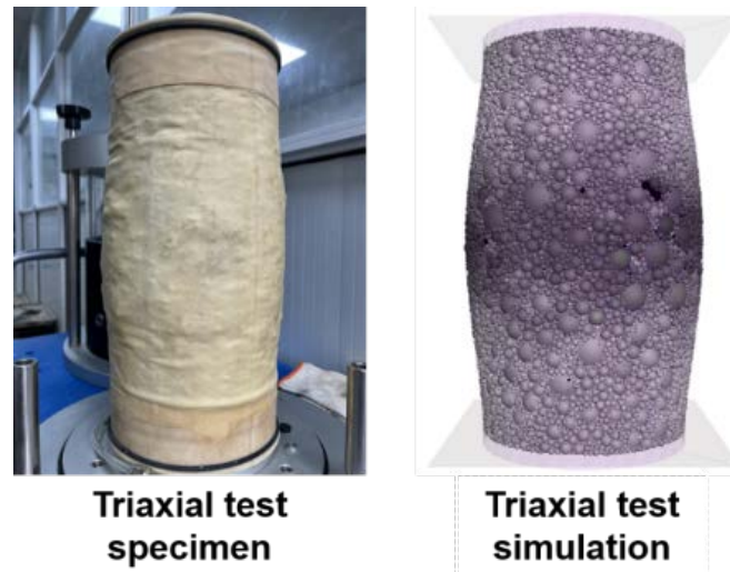
Figure 5: Triaxial shear test of unbound aggregates
