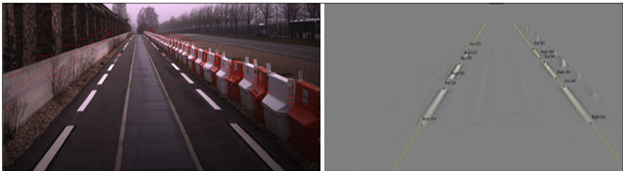
Figure 6: Real and final (enhanced) image to detect markings for contrast data
