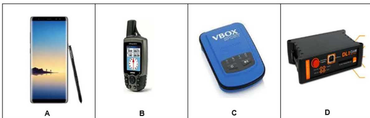
Figure 9: Onboard tracking devices: A – Mobile phone, B – Garmin handheld GPS, C – VBOX Sport GPS, and D – DL1 Club GPS
