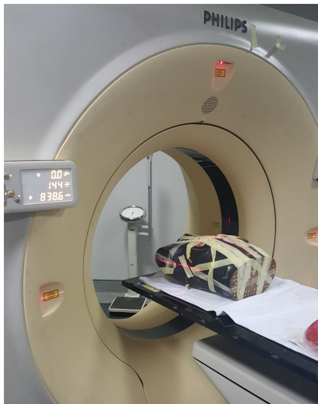
Figure 3.20 Scanning of the Rando phantom in the Big Bore CT scanner.
