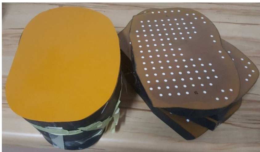
Figure 4.52 Radiochromic GafChromic films cut to the curvature of the Rando phantom and placed in-between the slices.
