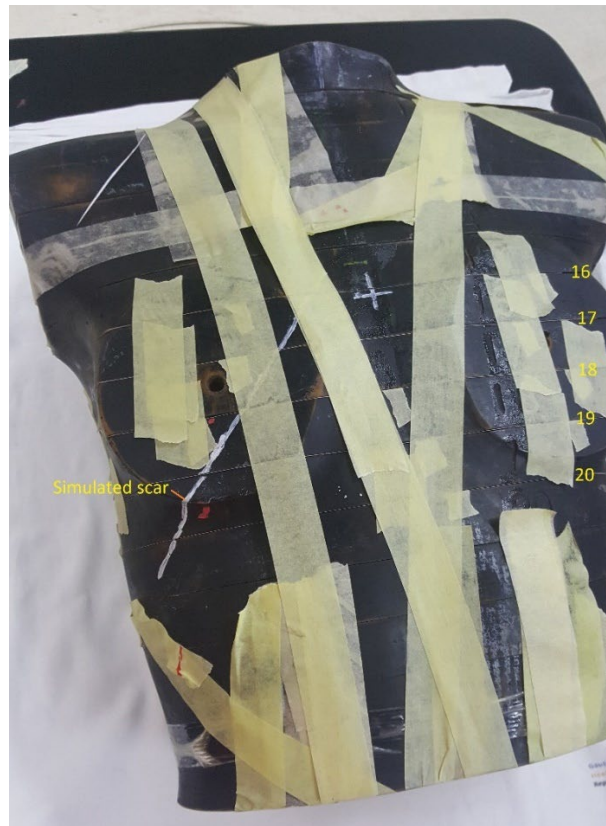
Figure 4.51 Rando phantom with a simulated scar and film slice position.
