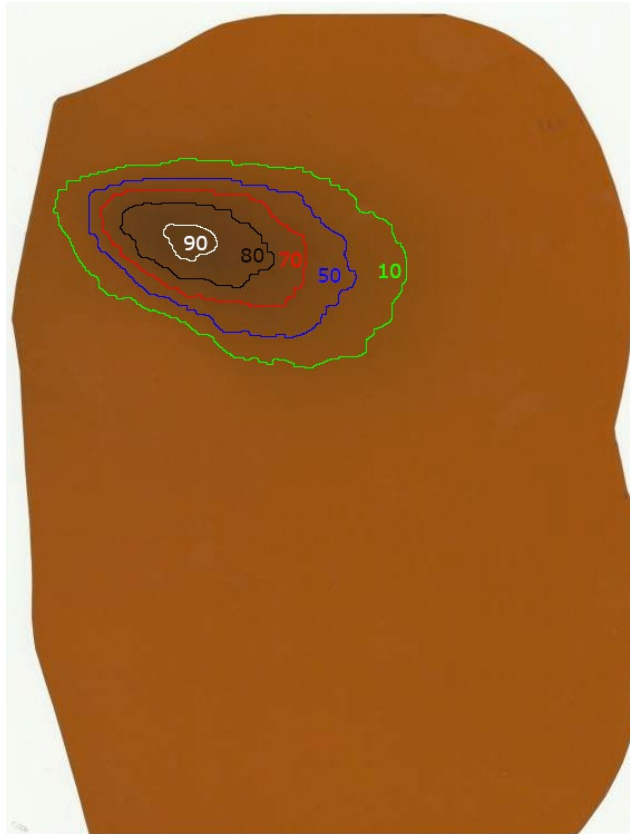
Figure 4.54 Scanned GafChromic films with isodose lines indicating the dose distribution. Films were at different positions of the Rando phantom: (a) is at position 16, (b) is at position 17, (c) is at position 18, (d) is at position 19, (e) is at position 20.
