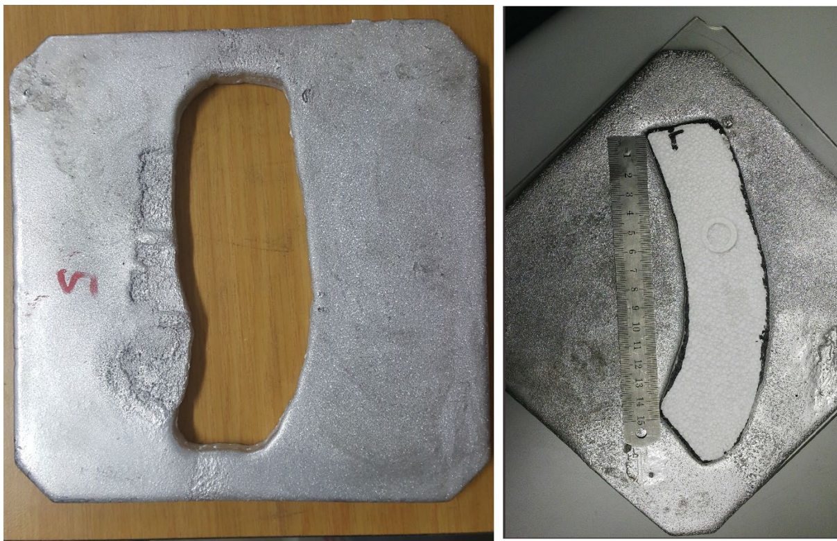
Figure 1.1 Typical electron cutouts made from Cerrobend that are used for the treatment of mastectomy scars.
