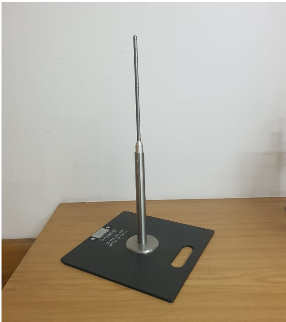
Figure 3.14 Pointer used to digitize that path to be followed by the couch.
