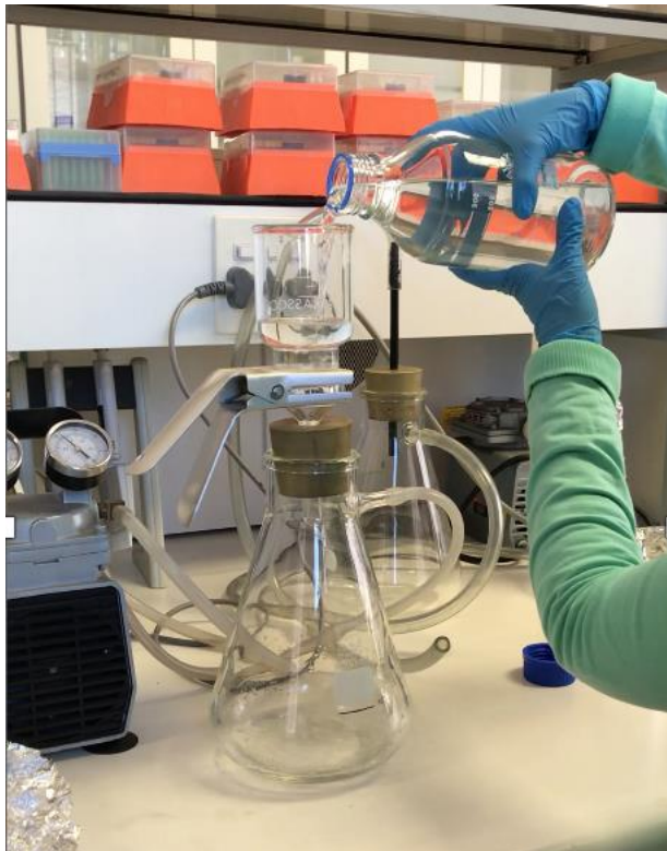
Figure 8: Glass Fibre Filter with Vacuum Pump to remove solid matter
