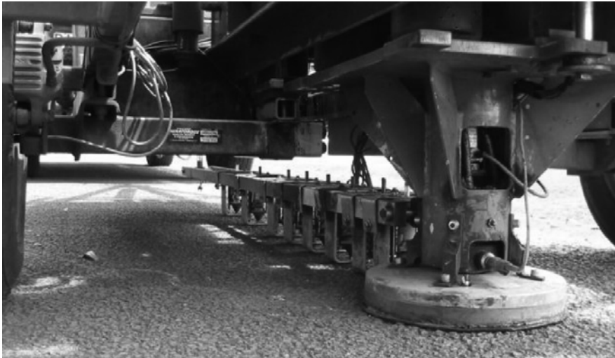
Figure 2. Falling weight deflectometer (FWD) configuration (Zheng et al. 2019).
