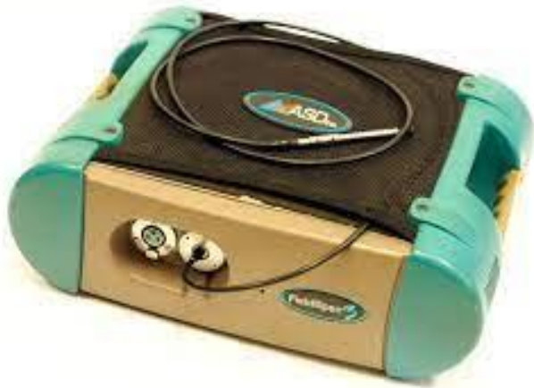
Figure 5: Fieldspec3; a device used to collect reflectance data, (Source: ASD Inc 2010).
