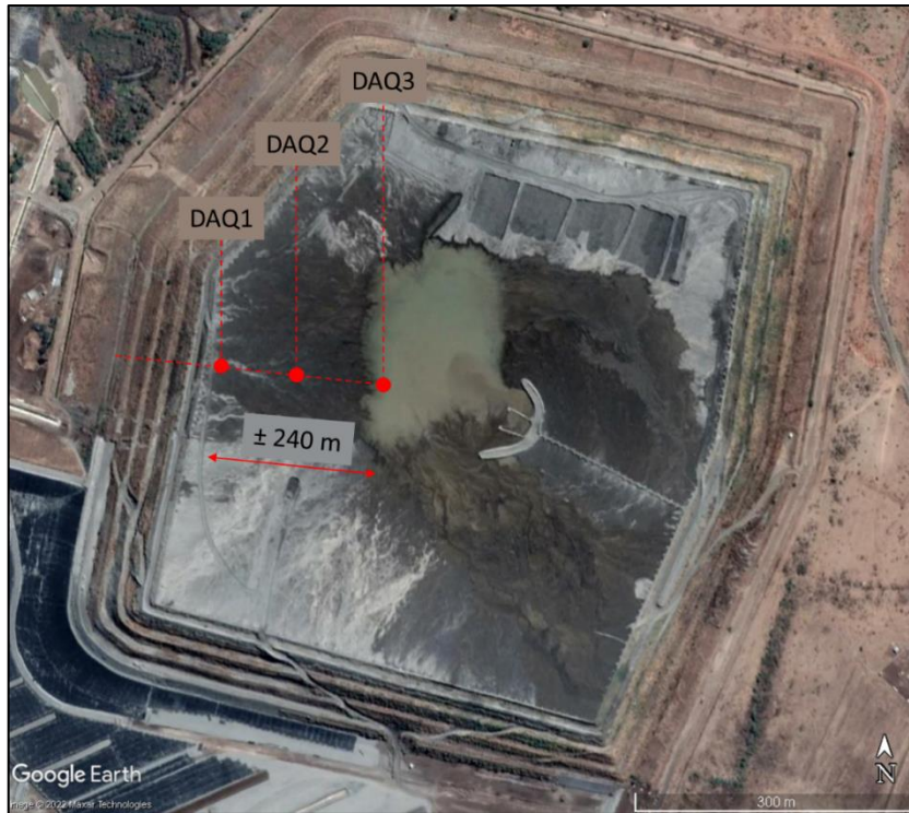
Figure 3.23: Data acquisition systems (DAQ) layout on a platinum tailings dam (Google Earth Pro, 2022).
