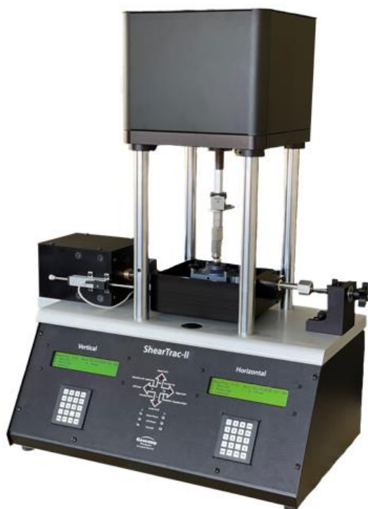
Figure 3.9: A Geocomp direct simple shear apparatus based on the NGI DSS (Geocomp, 2022).
