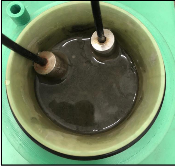
Figure 3.17: Tensiometers placed on top of a sample slurred into a membrane stretched over the DSS rings to monitor the generation of matric suctions during drying.
