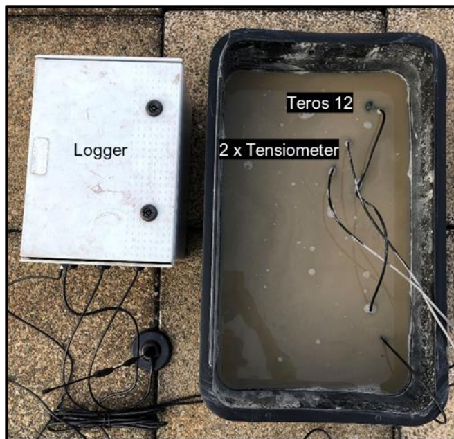
Figure 3.10: A 300mm x 600mm drying box filled with slurried platinum tailings instrumented with two tensiometers and one Teros 12 volumetric water content probe.
