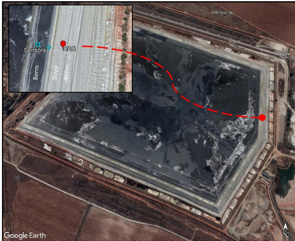
Figure 3.26: Data acquisition system position on a gold tailings dam (Google Earth Pro, 2022).
