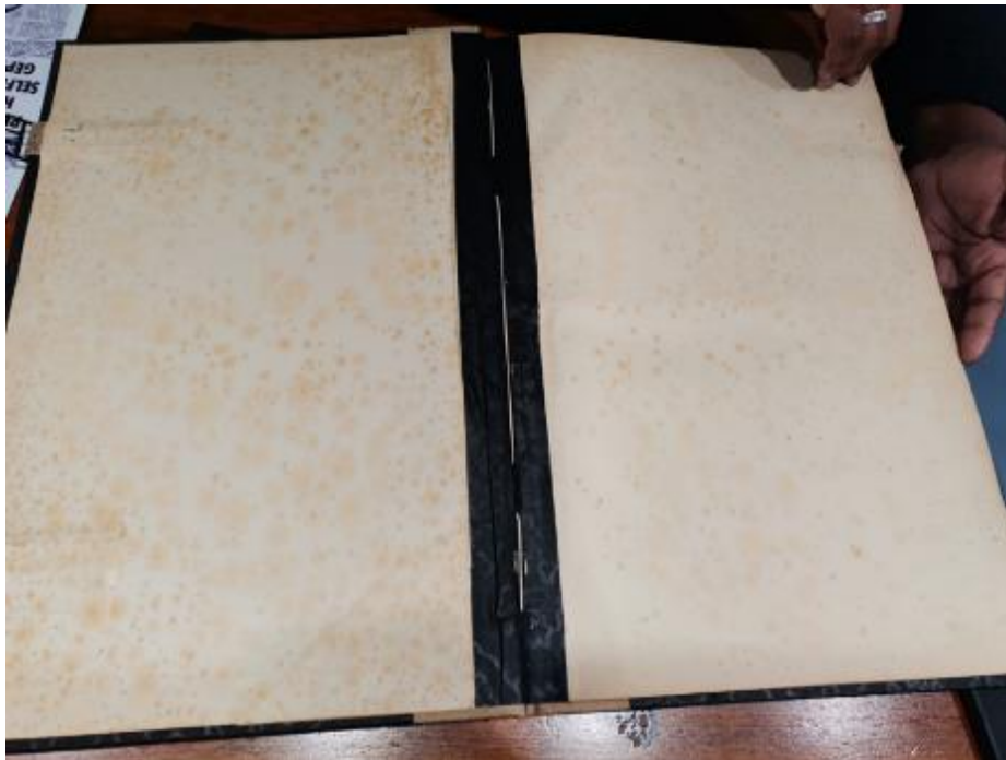
Figure 6: Insect damage from the cover of the publication and foxing 1931-1934 Moxwera publication, National Library of South Africa (Cape Town).
