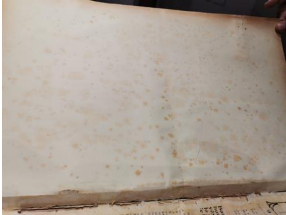
Figure 5: Foxing and insect damage on cover 1931-1934 Moxwera publication, NLSA (Cape Town).
