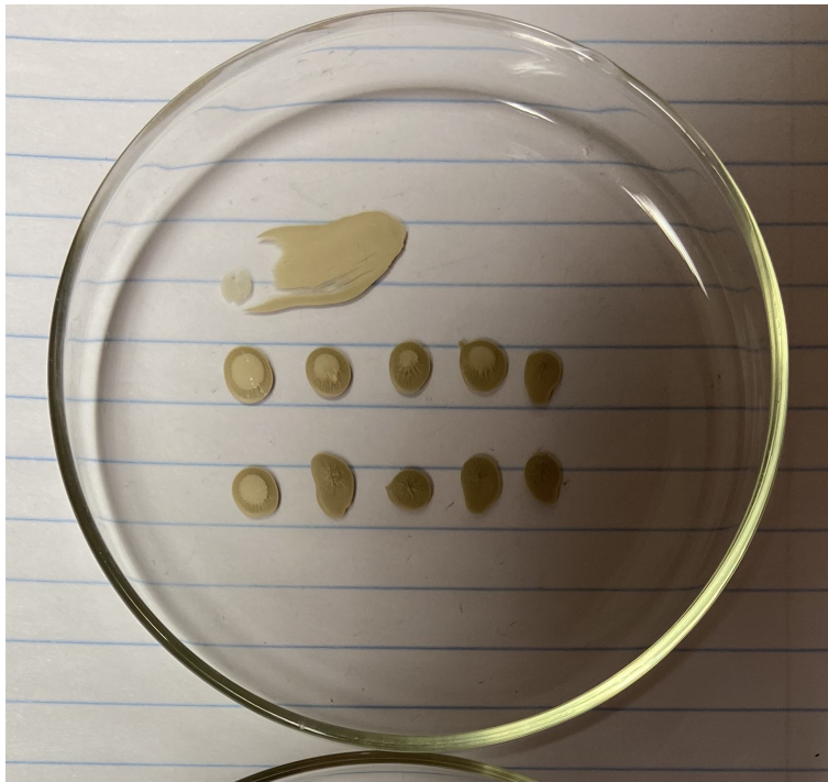
Figure 4.7. Drops mixed with resin and silver before curing.
