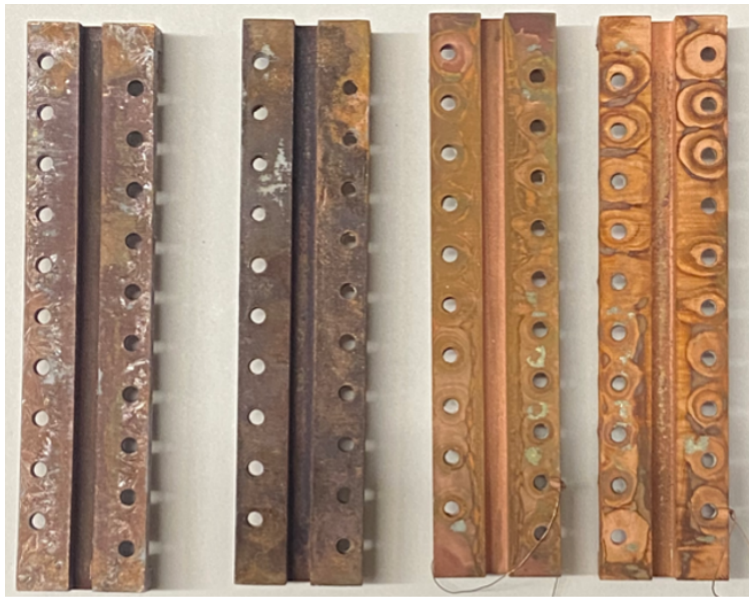
Figure 4.31. Corroded copper waveguide.
