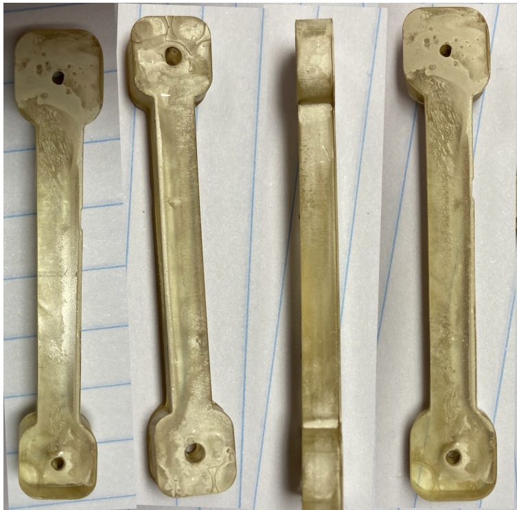
Figure 4.5. Conductive resin print with 50 % silver.
