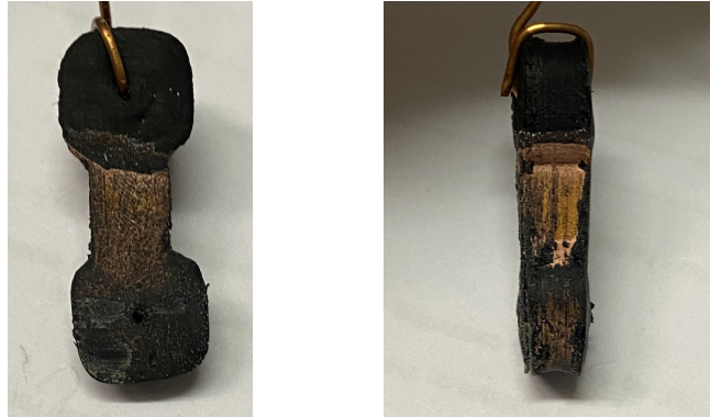
(a) Front view of the conductive FDM printing. (b) Side view of the conductive print where more copper formed.
