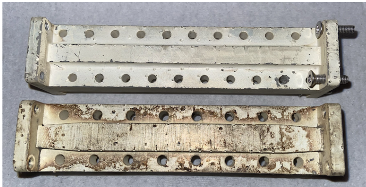
Figure 4.14. Dried waveguide (bottom) vs immersed and cooled waveguide (top).
