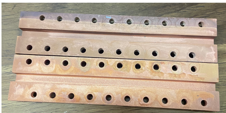
Figure 4.27. Waveguide after copper plating.
