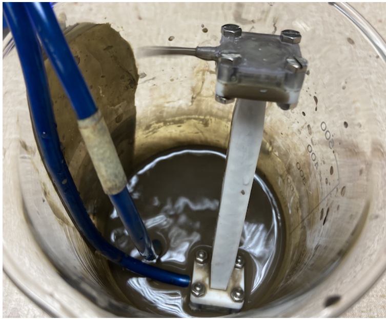
Figure 4.23. Waveguide being plated using a pump to move the plating solution.
