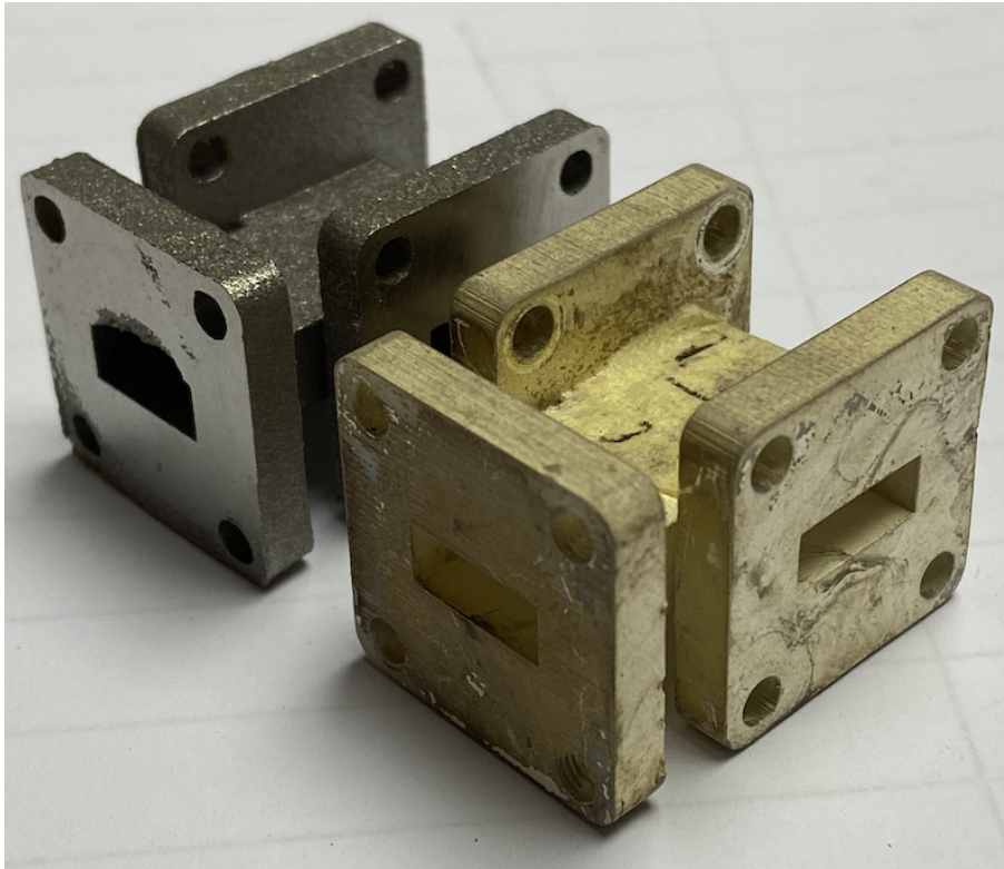
Figure 5.11. Manufactured SLA and SLM power dividers.
