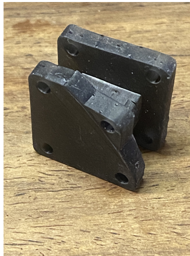
Figure 4.2. Waveguide with distorted flange due to insufficient support.
