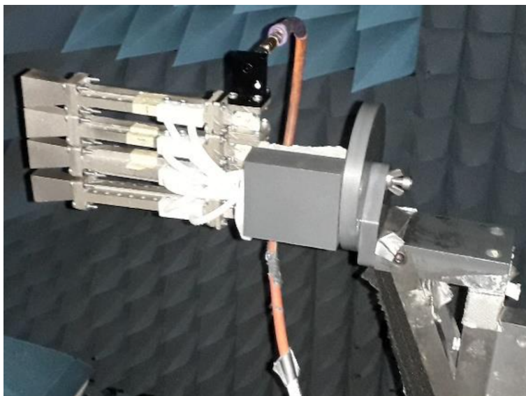
Figure 4.32. Metal antenna array during measurement.
