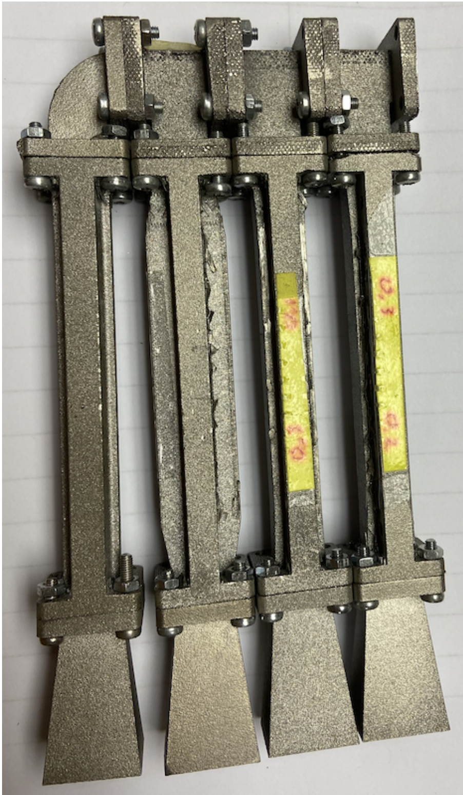
Figure 5.57. Assembled SLM horn array.
