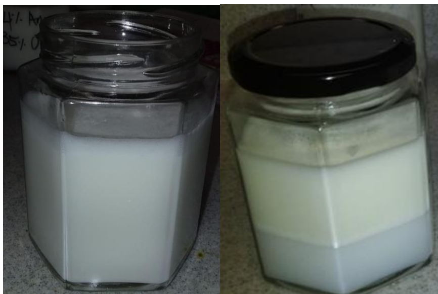
Figure 3.2: Homogeneous emulsion containing 5 wt.% surfactant just after preparation, (left) and after four weeks showing creaming (right)
