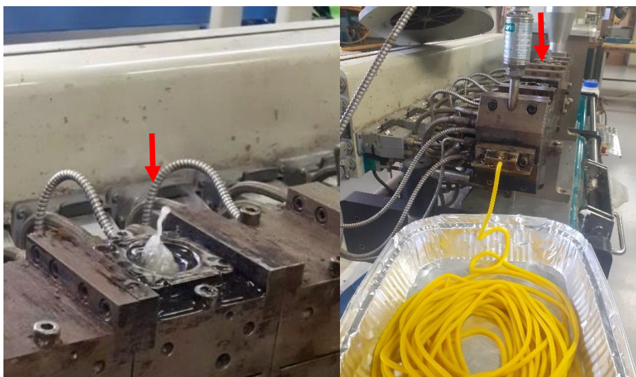
Figure 3.1: The white structure indicated by the arrow on the left is a fountain of liquid escaping from the vent due to the exudation of the oleic acid from the melt. This formulation did not contain any organoclay. On the right this effect was completely suppressed by the presence of 5 wt.% organoclay in the formulation
