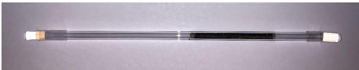
Figure S1: Graphene wool sampler showing the GW of 60 mm bed length housed in a glass tube with glass end caps held in place by Teflon sleeves. Source: Adapted from (Schoonraad and Forbes, 2019b).
