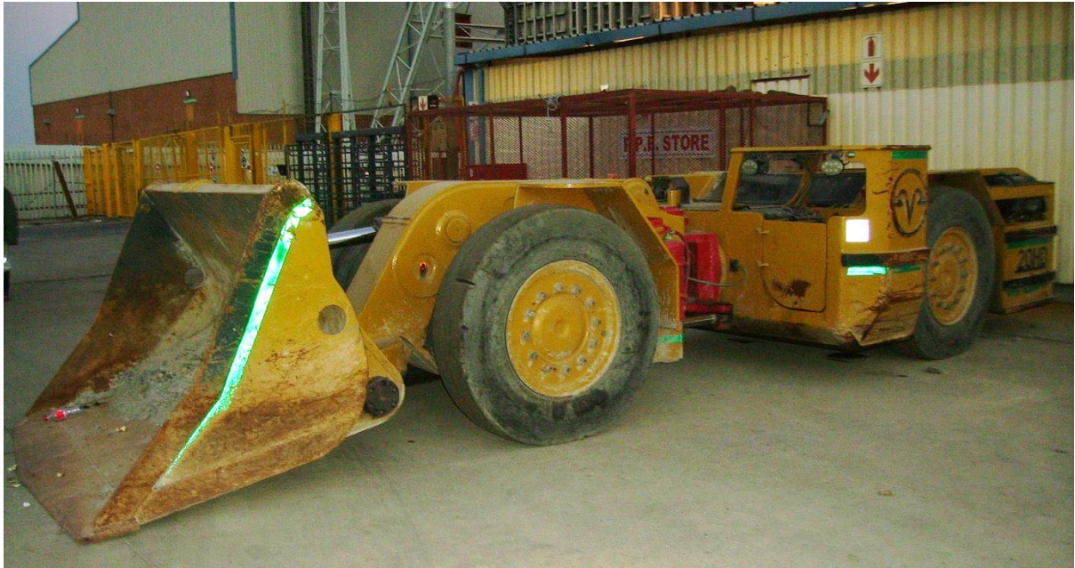
Figure S1 Photograph of load haul dump vehicle used for underground mining operations
