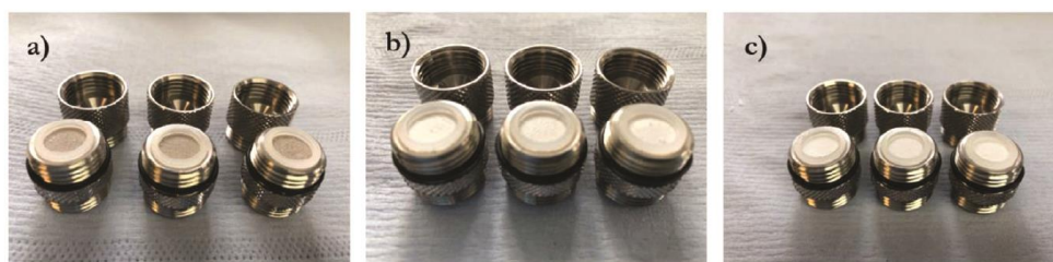
Fig. 5. PM filtered from (a) B0, (b) GTL and (c) RME CAST emissions prior to gas phase sampling.
