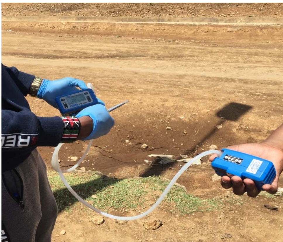
Figure S5. Collection of ambient air samples by the untarred roadside (sampling trap was held at 100 cm above the ground).
