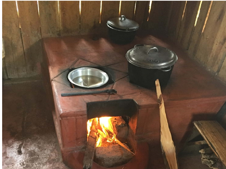
Figure S2. Typical improved 3-stone stove molded with bricks and cement.
