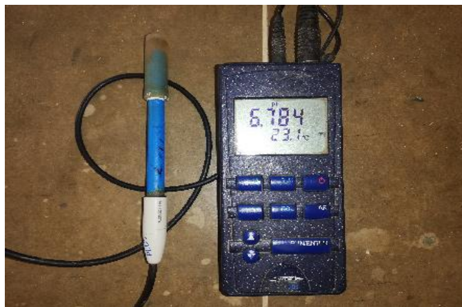
Figure 3.8 Handheld pH meter (WTW pH240i pH meter/data logger attached with a WTW Sentix 41 pH electrode)
