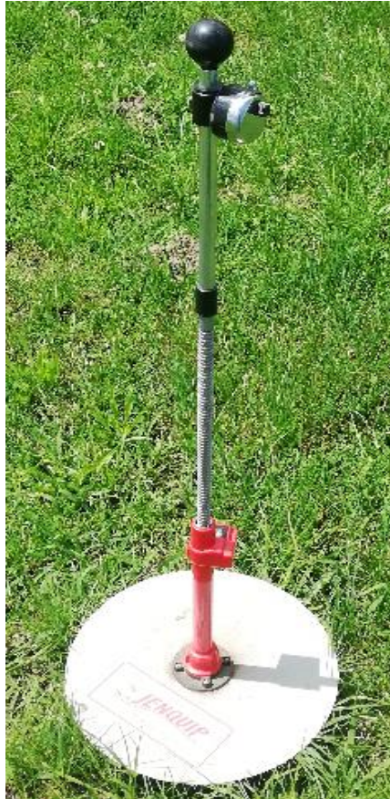
Figure 3.3 Rising plate meter used to measure pre- and post-grazing heights and to determine seasonal regression equations
