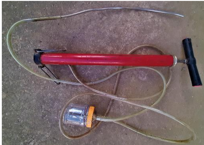
Figure 3.10 Customised hand pump used for rumen fluid collection via the rumen cannula
