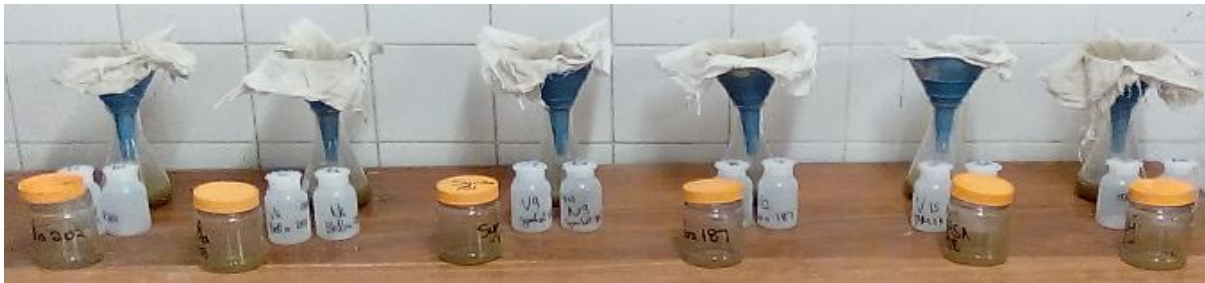
Figure 3.11 Rumen fluid collected, filtered through four layers of cheesecloth and divided into two 25ml sample bottles for VFA and ruminal ammonia nitrogen analysis respectively
