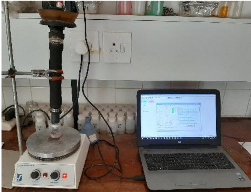
Figure 3.7 Indwelling pH logger calibration with Omnilog data management program
