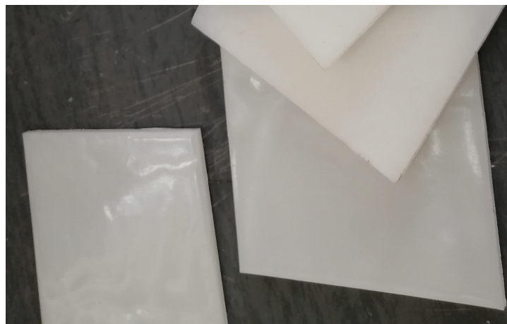
Figure 5.3: Example of the wavy or rippled surface observed for UP compression moulded samples.
