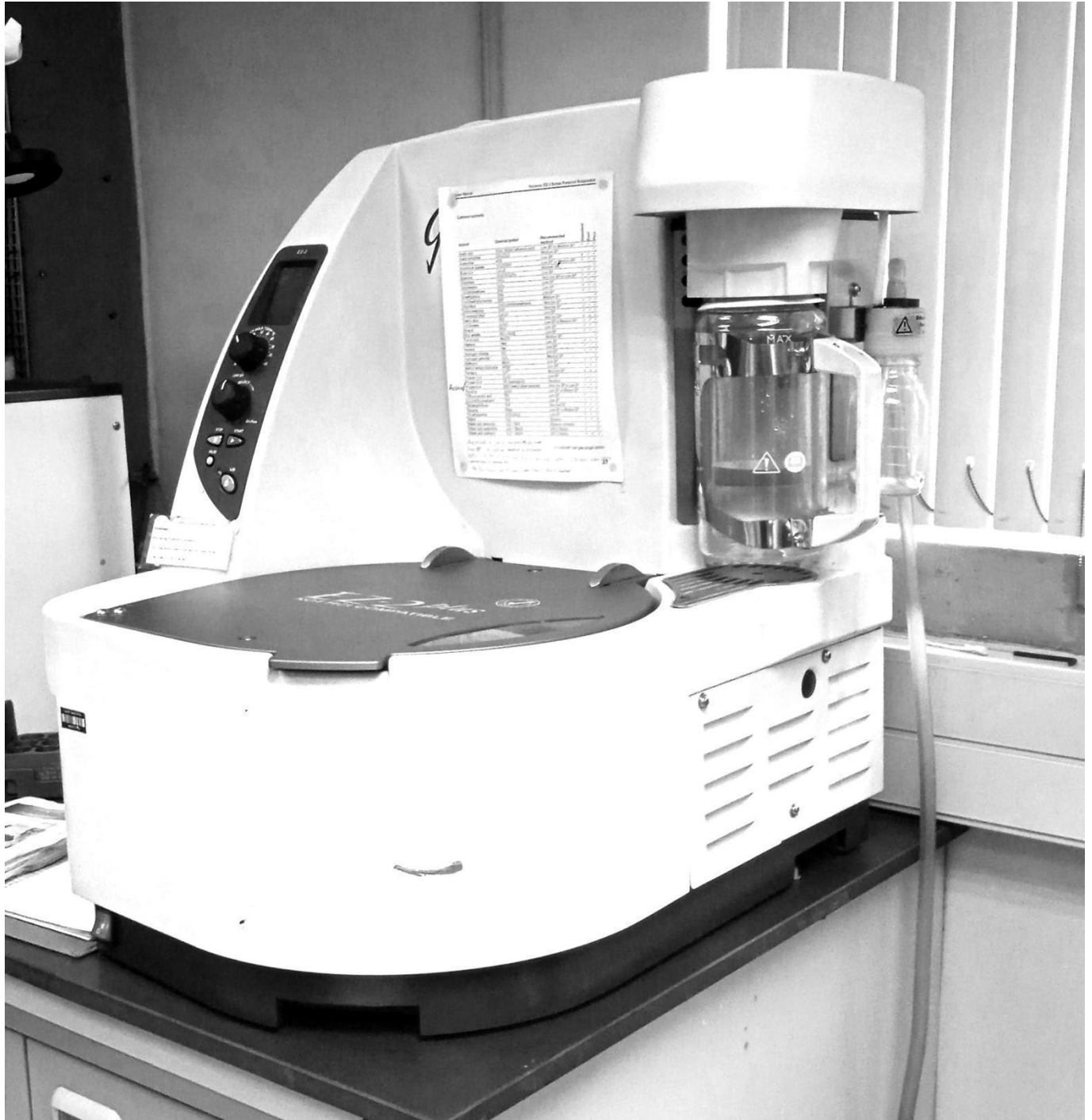
Figure 3.1 The Genevac (EZ-2 series, SP Scientific, England) used to separate the broth from bacterial supernatant as well as drying the methanolic extracts
