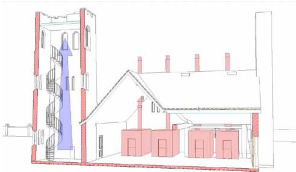
Figure 81: Section through furnace hall & bell tower suggesting new placement, within bell tower, of heat capture/energy generation systems for augmentation.
