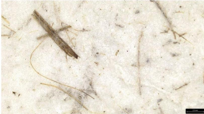
Figure 84: White rhinoceros' dung paper after 2 weeks of UV radiation (x 2) (2,5mm). Photo: Leica S9i microscope (2022).
