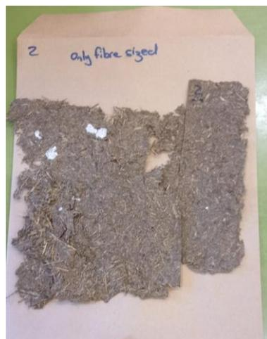
Figure 55: Paper samples made of rhinoceros' dung, only fibre and it was sized. Photo: Author (2022).
