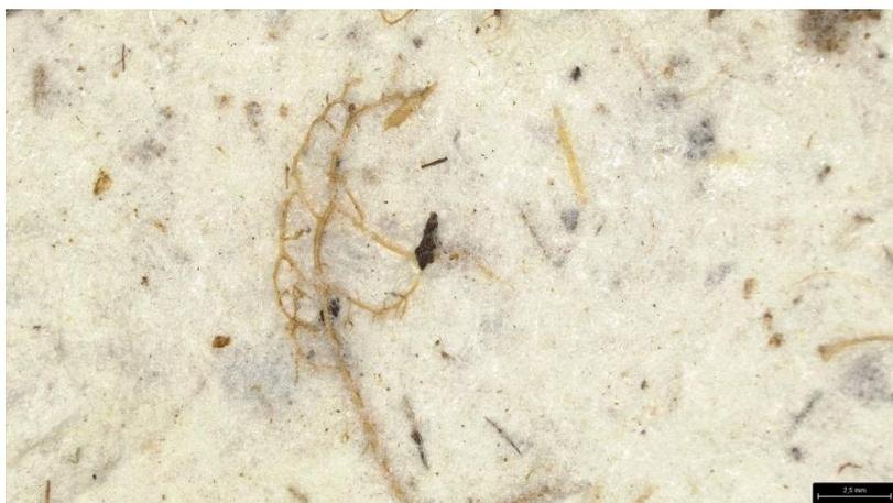
Figure 81: Kruger elephant dung paper after 4 weeks of UV radiation (x 2) (2,5mm). Photo: Leica S9i microscope (2022).
