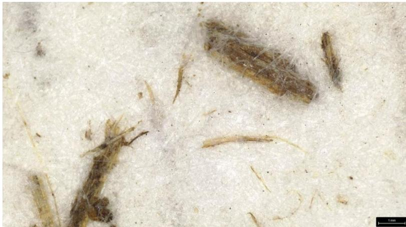
Figure 85: White rhinoceros' dung paper after 4 weeks of UV radiation (x 2) (1mm). Photo: Leica S9i microscope (2022).
