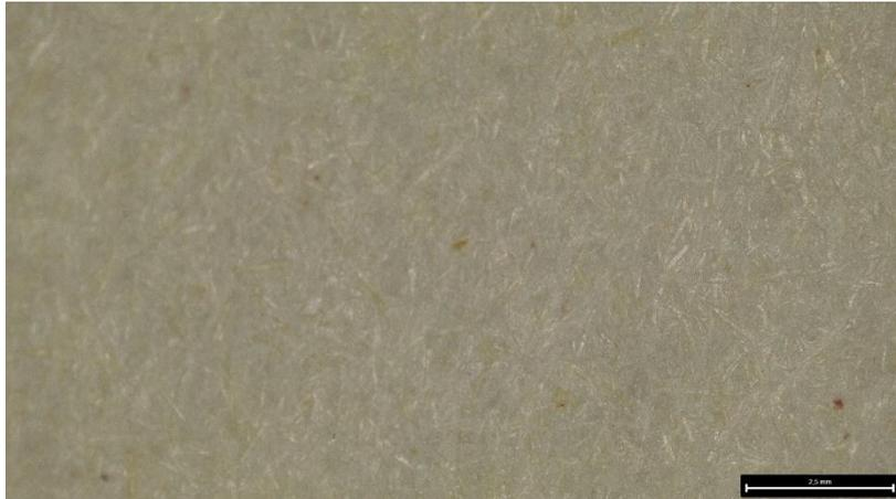
Figure 91: Newsprint paper before UV testing at day 0 (x 2) (2,5mm). Photo: Leica S9i microscope (2022).
