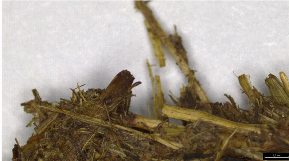
Figure 95: Unsized rhinoceros' dung made paper with coarser fibres shows the pulling out of fibres rather than the breaking of fibres (2,5 mm). Photo: Leica S9i microscope (2022).
