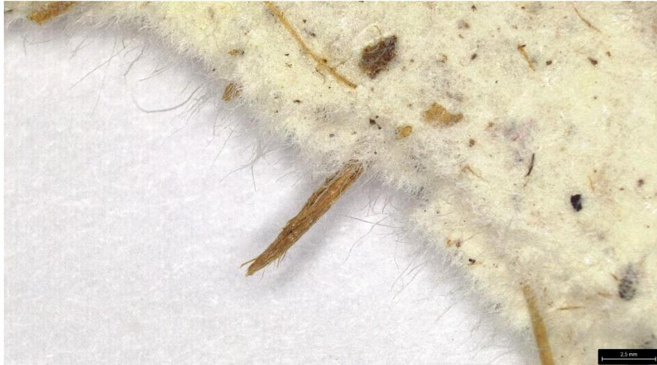
Figure 99: Kruger elephant dung made paper shows how the finer bonded fibres tore, while the coarser fibres pulled out at the tear (2,5 mm). Photo: Leica S9i microscope (2022).
