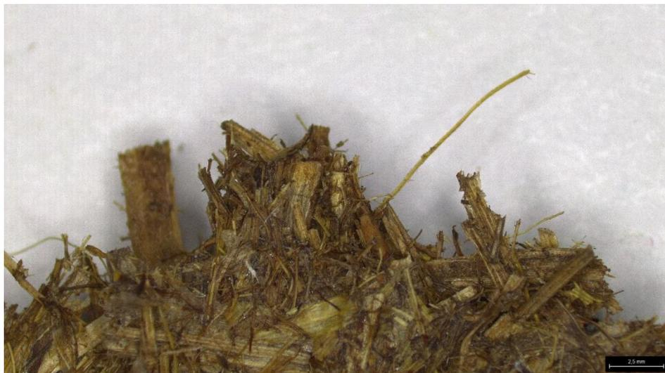
Figure 96: Sized rhinoceros' dung made paper shows the similar effect of fibres that pulled out rather than broke (2.5 mm). Photo: Leica S9i microscope (2022).
