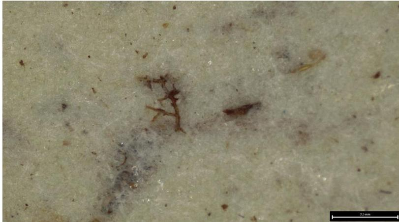
Figure 79: Kruger elephant dung paper before testing (day 0) (x 2) (2,5mm). Photo: Leica S9i microscope (2022).
