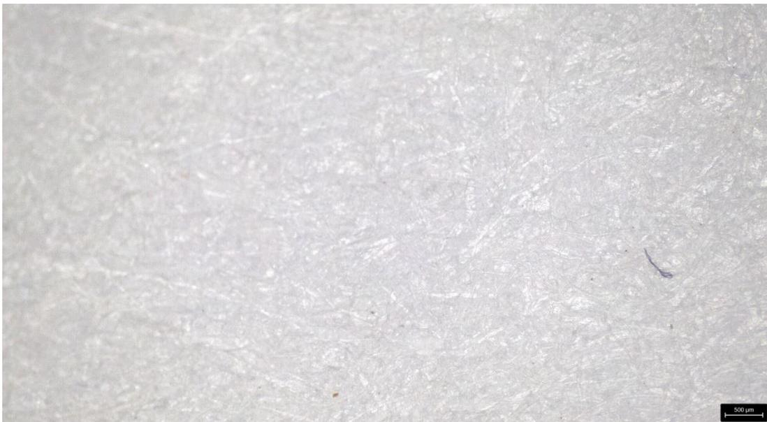
Figure 78: Sappi paper after 4 weeks of UV radiation (x 2) (500 μm). Photo: Leica S9i microscope (2022).
