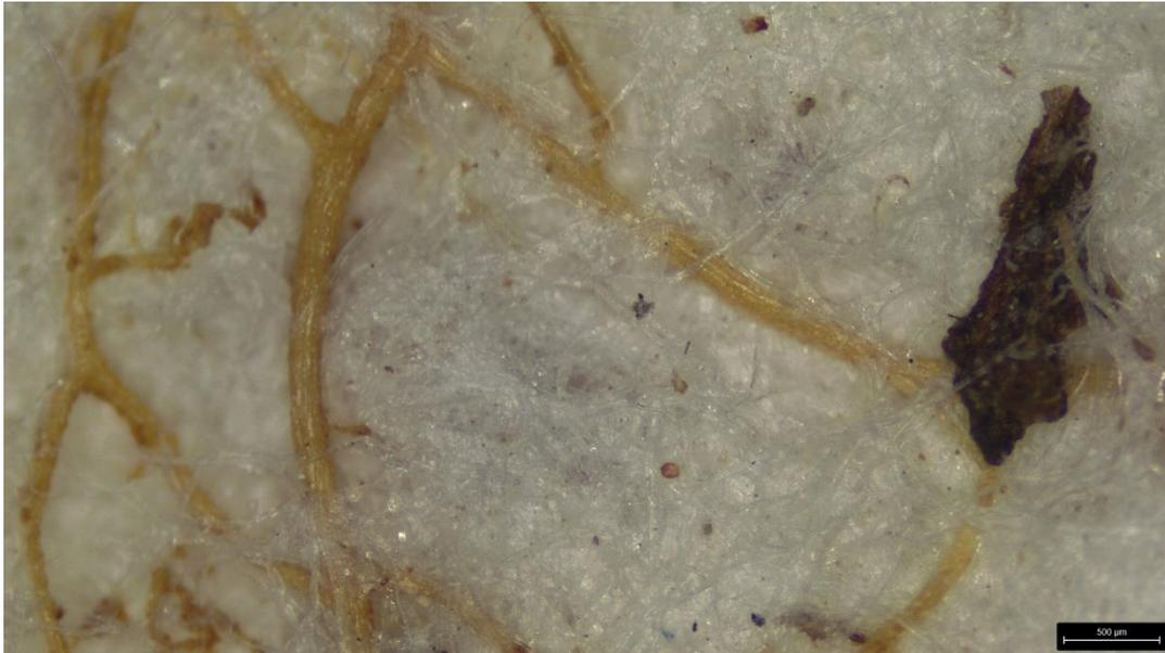
Figure 82: Kruger elephant dung paper after 4 weeks of radiation with no sign of fibre degradation (x 4) (500 µm). Photo: Leica S9i microscope (2022).
