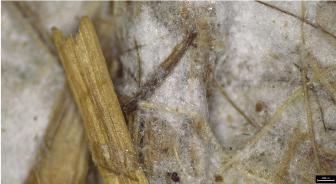
Figure 75: Rhinoceros' dung and Sappi paper after 4 weeks of UV radiation with no indication of fibre degradation (x 4) (500 µm). Photo: Leica S9i microscope (2022).
