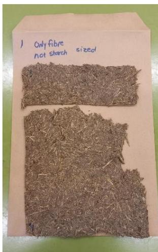
Figure 54: Paper made of rhinoceros' dung, only fibre and not sized. Photo: Author (2022).
