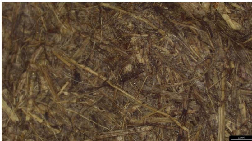
Figure 71: Paper of rhinoceros dung fibre (sized) after 4 weeks of UV radiation (x 2) (2,5mm). Photo: Leica S9i microscope (2022).
