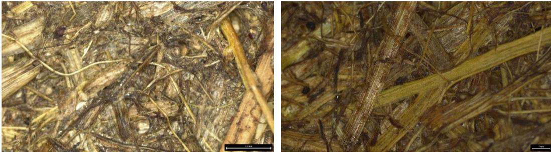
Figure 46: Rhinoceros' dung paper, not sized, before (left) and after absorption (left). No mold or any other growth was observed. Photo: Leica S9i microscope (2022).
