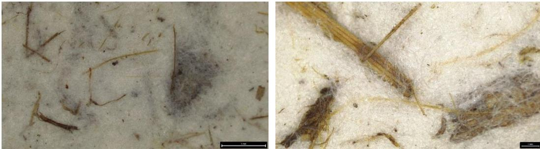
Figure 51: White rhinoceros' dung paper before (left) and after (right) absorption. No mold or any other growth was observed. Photo: Leica S9i microscope (2022).
