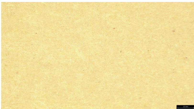
Figure 93: Newsprint paper after 4 weeks of UV radiation (x 2) (2,5mm). Photo: Leica S9i microscope (2022).
