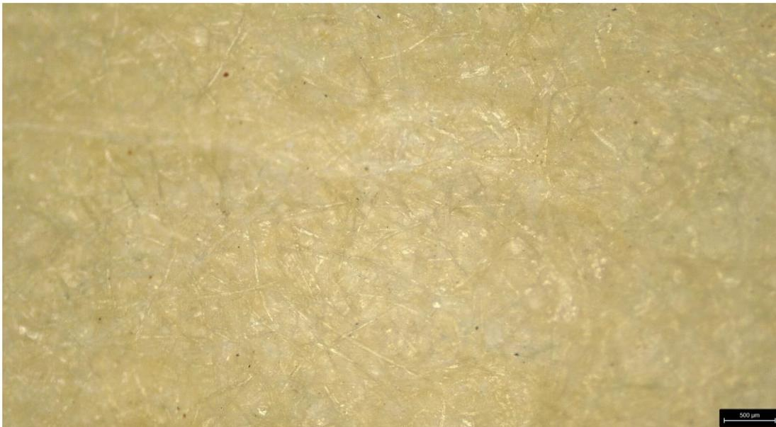
Figure 90: Chinese artist paper after 4 weeks of UV radiation with no signs of fibre degradation, but a pink to brownish discolouring (x 4) (500 µm). Photo: Leica S9i microscope (2022).
