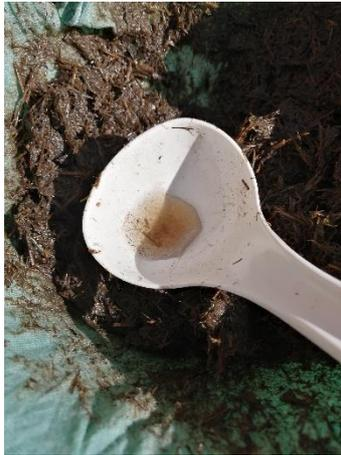
Figure 22: Washing the pulp until the water is near clear. Photo: Author (2022).
