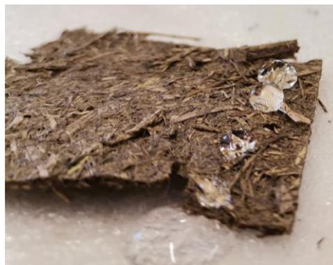
Figure 30: Black rhinoceros' dung paper (sized) with droplets of distilled water. Photo: Author (2022).
