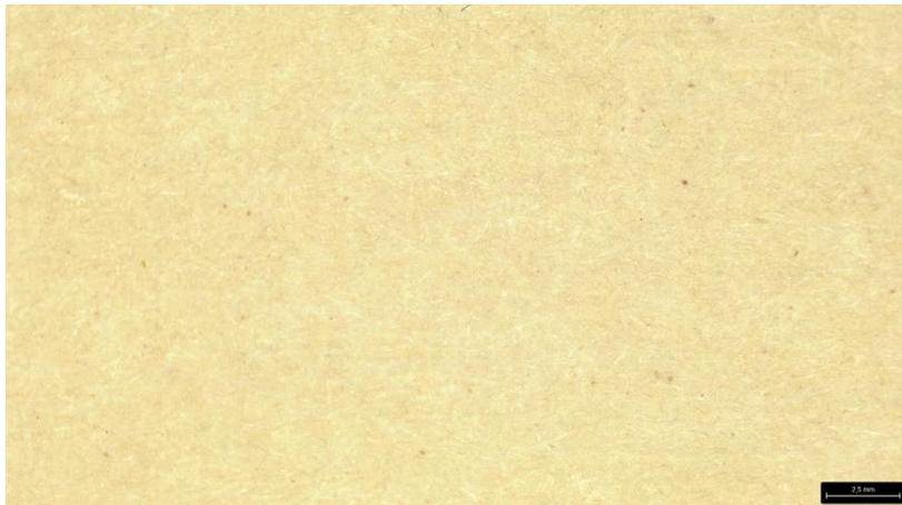
Figure 92: Newsprint paper after 2 weeks of UV radiation (x 2) (2,5mm). Photo: Leica S9i microscope (2022).
