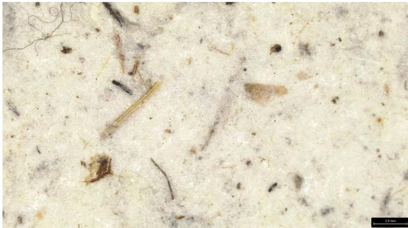
Figure 80: Kruger elephant dung paper after 2 weeks of UV radiation (x 2) (2,5mm). Photo: Leica S9i microscope (2022).
