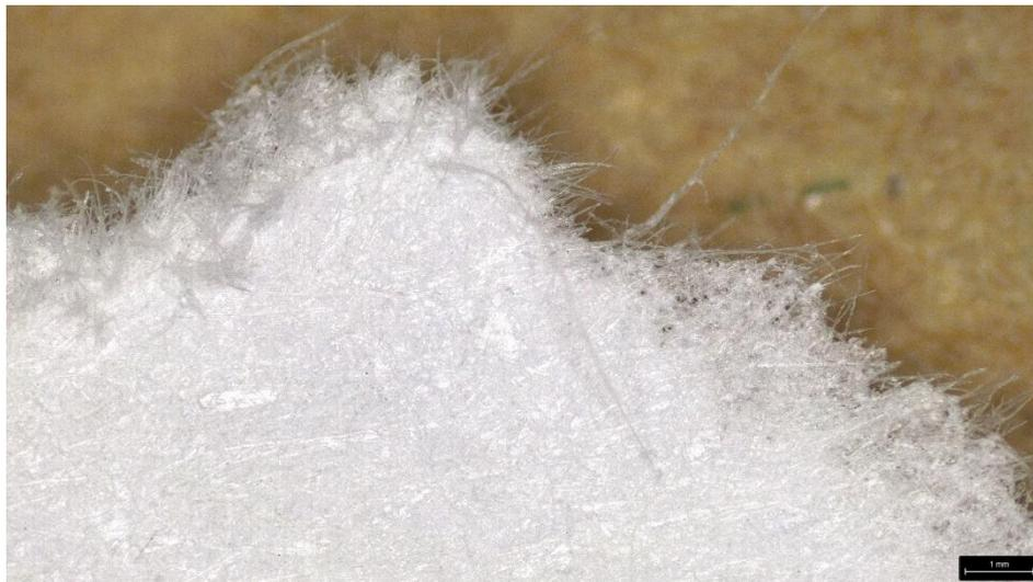
Figure 98: Sappi paper shows how the finer bonded fibres tore (1 mm). Photo: Leica S9i microscope (2022).
