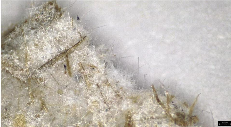
Figure 97: Rhinoceros' dung with Sappi paper shows the finer bonded fibres of the Sappi paper that tore while the coarser fibres pulled out (500 µm). Photo: Leica S9i microscope (2022).
