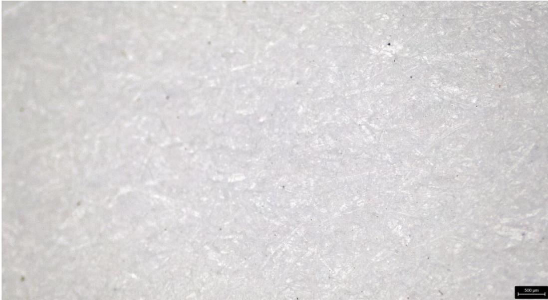
Figure 77: Sappi paper after 2 weeks of UV radiation ((x 2) 500 μm). Photo: Leica S9i microscope (2022).
