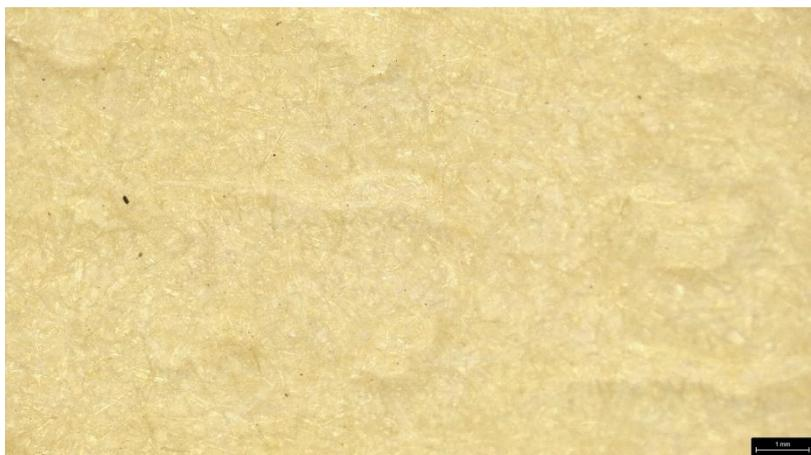
Figure 89: Chinese artist paper after 4 weeks of UV radiation (x 2) (1mm). Photo: Leica S9i microscope (2022).
