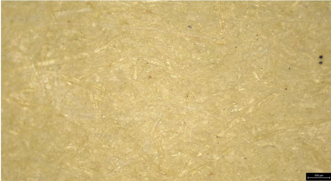
Figure 94: Newsprint after 4 weeks of UV radiation with no fibre degradation, but a pink to brownish discolouring (x 4) (500  $\mu\text{m}$ ). Photo: Leica S9i microscope (2022).
