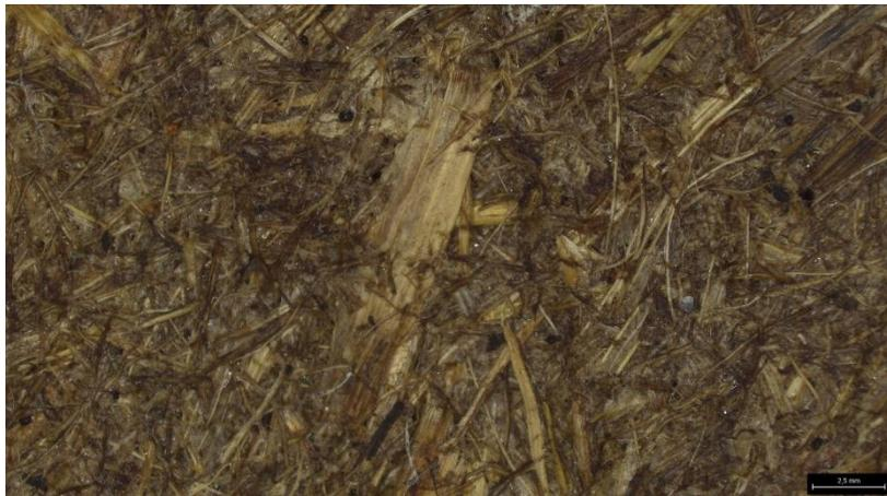
Figure 70: Paper of rhinoceros dung fibre (sized) after 2 weeks of UV radiation (x 2) (2,5mm). Photo: Leica S9i microscope (2022).
