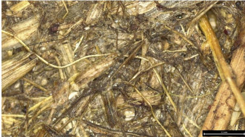
Figure 66: Paper of rhinoceros dung fibre (not sized) before testing (day 0) (x 2) (2,5mm). Photo: Leica S9i microscope (2022).
