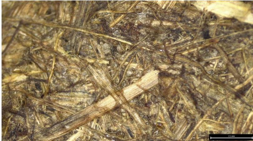
Figure 69: Paper of rhinoceros fibre (sized) before testing at day 0 (x 2) (2,5mm). Photo: Leica S9i microscope (2022).
