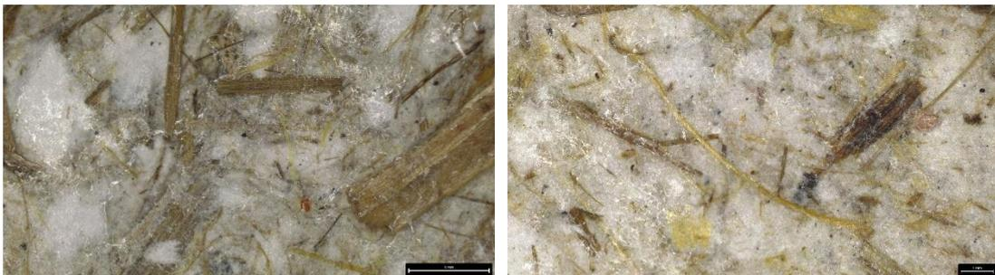
Figure 48: Rhinoceros' dung and Sappi paper before (left) and after (right) absorption. No mold or any other growth was observed. Photo: Leica S9i microscope (2022).
