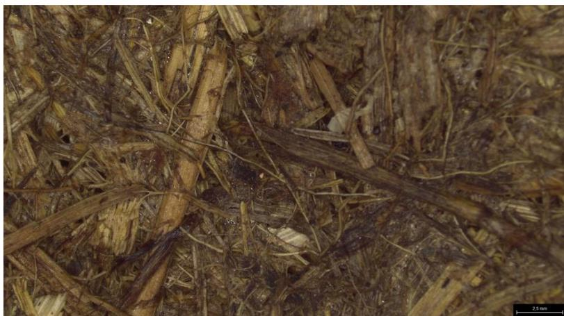
Figure 68: Paper of rhinoceros dung fibre (not sized) after 4 weeks of UV radiation (x 2) (2,5mm). Photo: Leica S9i microscope (2022).
