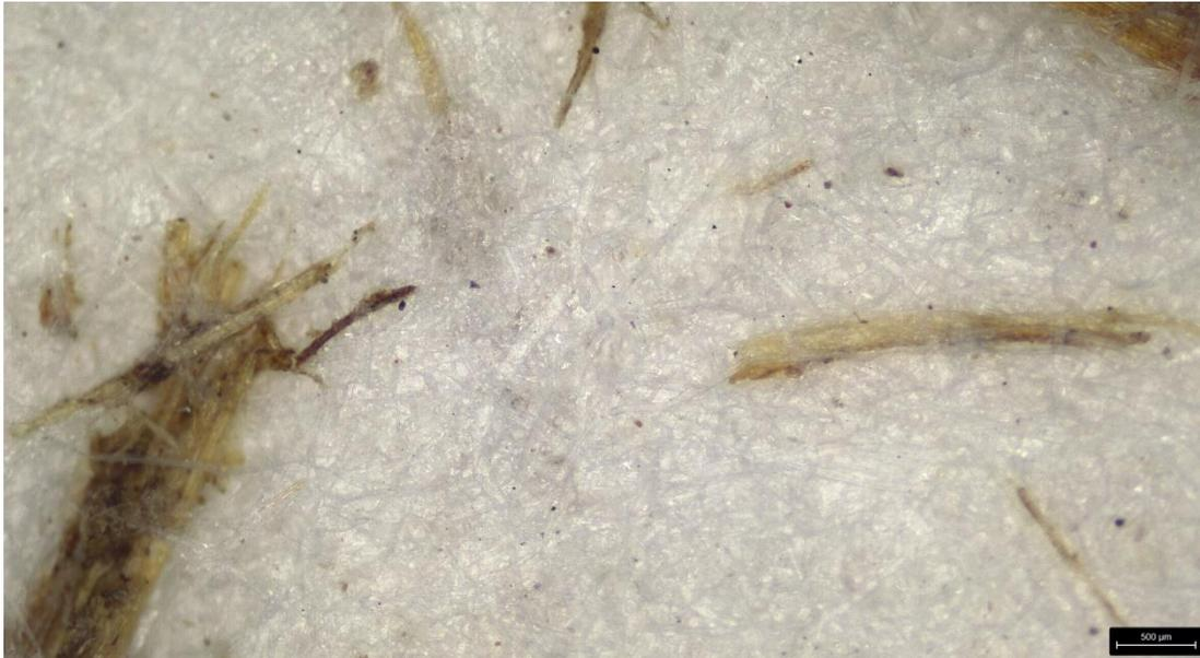
Figure 86: White rhinoceros' dung paper after 4 weeks of UV radiation with no sign of fibre degradation (x 4) (500 µm). Photo: Leica S9i microscope (2022).
