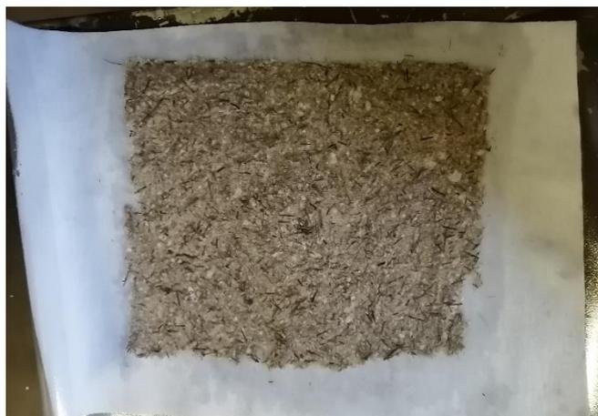
Figure 26: Sheet couched onto felt and plastic sheet. Photo: Author (2022).
