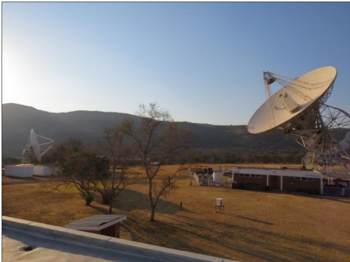
Figure 4.1 The Stevenson screen on the lawn in the foreground houses the temperature and humidity sensors for astrometric and geodetic VLBI.
