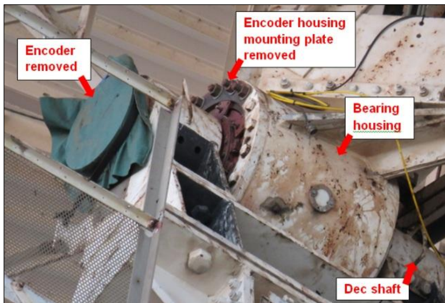
Figure 3.3 HartRAO 26 m antenna west end of declination shaft with encoder removed. Photo credit: J. Grobler.
