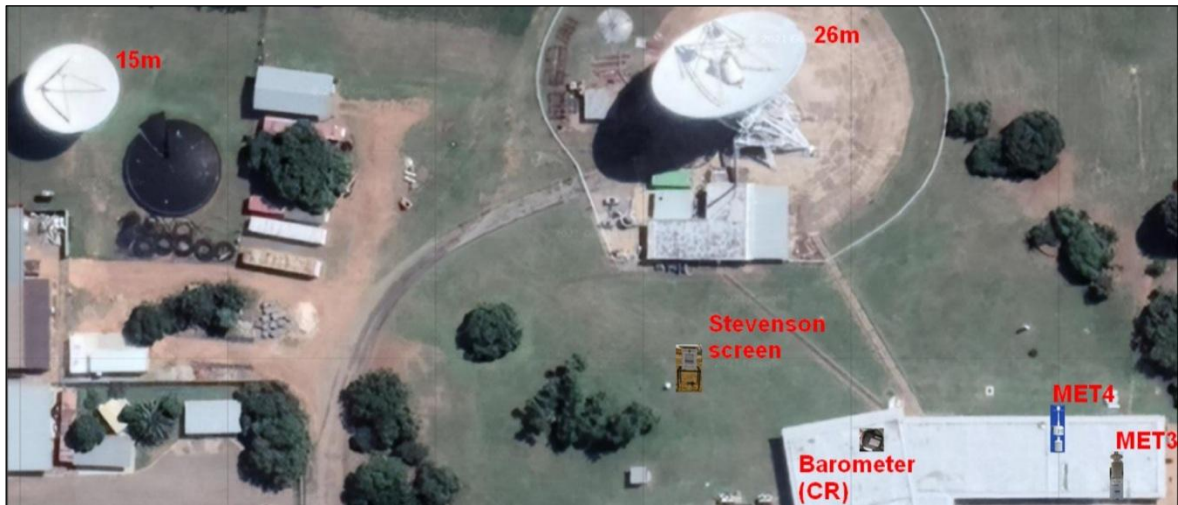
Figure 4.2 Location of HartRAO meteorological sensors and MET3 and MET4 units with respect to the 15 m and 26 m antennas.
