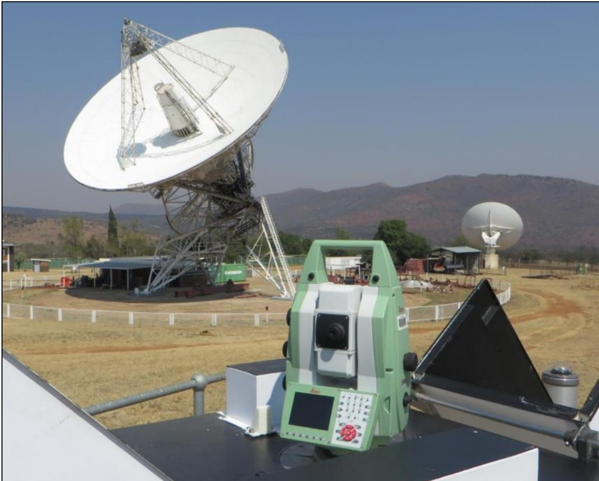
Figure 7.1 Short baseline of ~113 m between the HartRAO 26 m and 15 m antennas with the total station (Leica MS50 Multistation) under test in the foreground. Photo credit: R. Botha.
