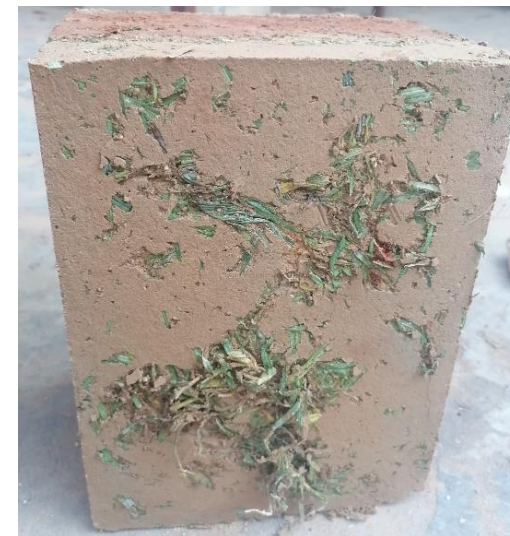
Fig 181: 70% soil, 15% grass and 15% concrete (Author 2022).
