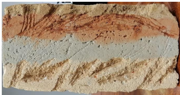
Fig 179: 70% soil and 30% concrete and carved by hand (Author 2022).
