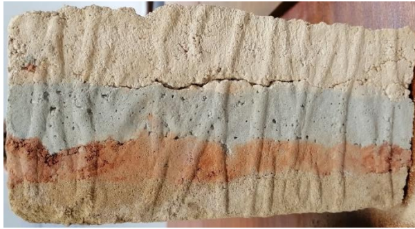
Fig 177: 70% soil and 30% concrete with carved form work (Author 2022).
