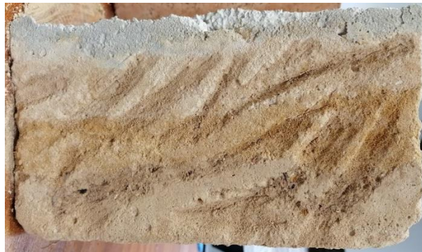
Fig 178: 90% soil and 10% concrete smooth framework and carved by hand (Author 2022).
