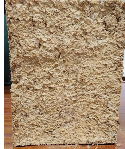
Fig 180: 70% soil, 15% grass and 15% concrete with woodchips in concrete mixture (Author 2022).
