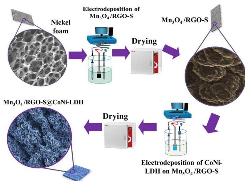
FIGURE 1 Schematic illustration of the synthesis of Mn<sub>3</sub>O<sub>4</sub>/RGO-S@CN electrode
