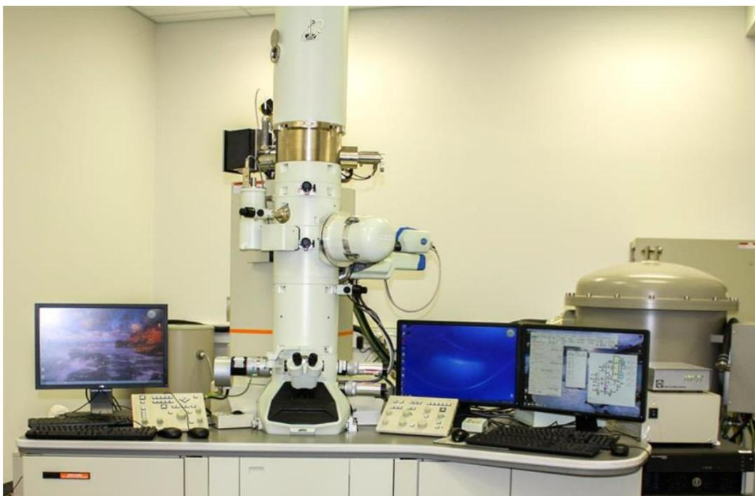
*Figure 3.10: Transmission electron microscope (JEOL JEM-2100F).*
