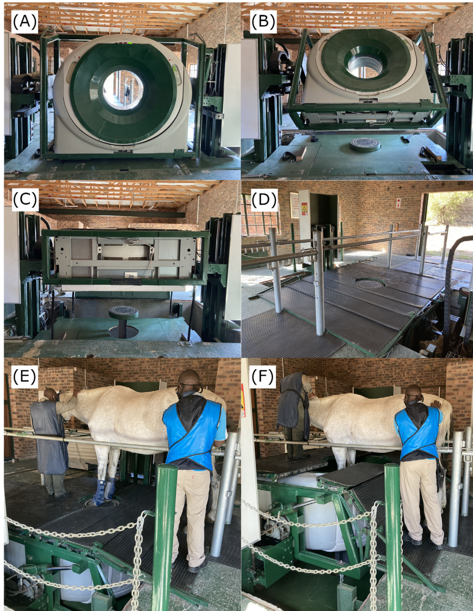
FIGURE 1 Helical 128-slice prototype CT scanner mounted on hydraulics used in this study. A, The 72 cm bore diameter gantry protected by a metallic shield in a vertical position. B, Gantry being tilted to a horizontal position. C, Gantry in a horizontal position being lowered until floor level into a pit. D, CT scanner ready for distal limb acquisition in the standing horse. A rubber floor cover protects the horizontally placed gantry. Stocks are in place. E, Pre-CT scan image showing the sedated horse positioned for examination of the front limbs. These are placed on a pedestal in the middle of the gantry. Notice the placement of the two handlers. F, Image obtained during CT acquisition of the front limbs. The gantry moves vertically along the horse's limbs [Color figure can be viewed at wileyonlinelibrary.com ]
