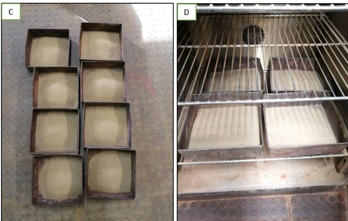
Figure 3.4: C: soil samples after splitting; D: Oven-drying soil samples
