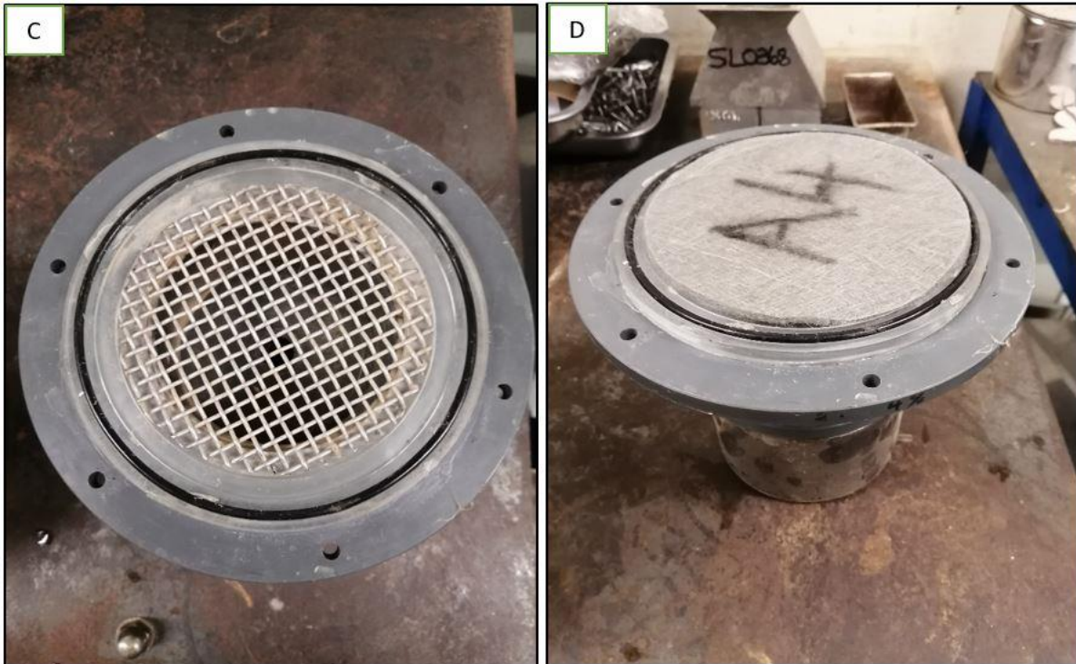
Figure 3.7: C: support screen in position prior to geotextile placement. D: Geotextile on top of support screen
