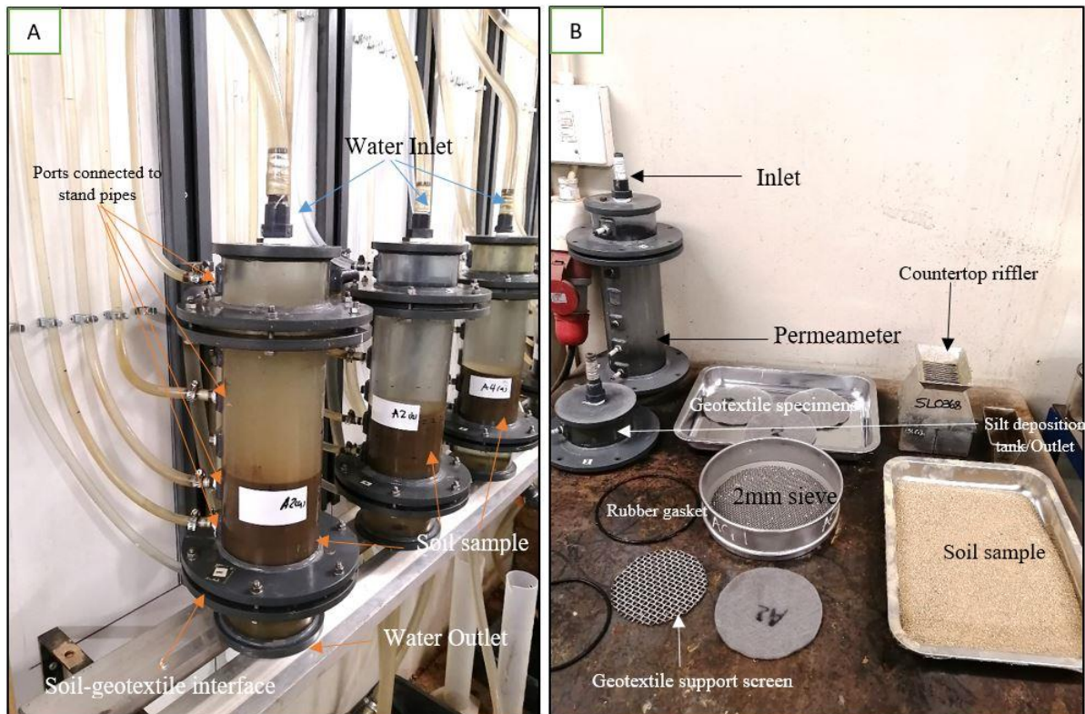
Figure 3.5 A: LTGR Setup during testing; B: LTGR components, riffler, soil and geotextiles samples.
