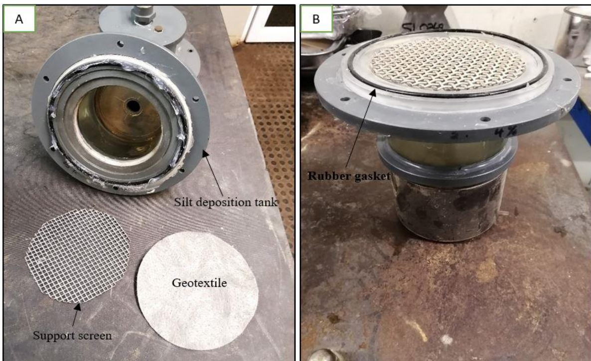
Figure 3.6: A: Silt deposition tank, support screen and geotextile. B: Silt deposition tank with support screen on top
