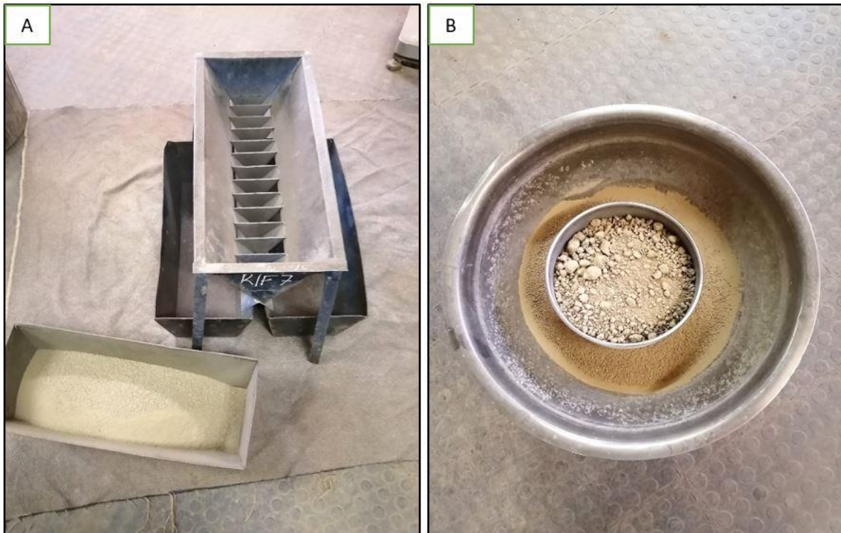
Figure 3.3: Sample preparation: A: Soil sampling splitting; B: Sieving with 2 mm sieve
