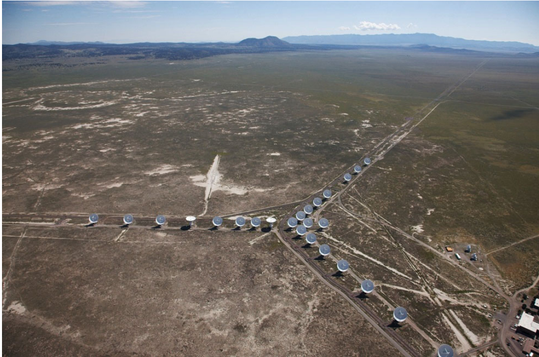
FIGURE 1.9: The VLA antenna layout. The antennas are arranged in a Y configuration to allow for a variety of reasons, as explained in the text. Credit: NRAO.
