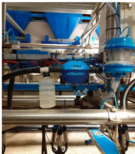
Figure 3-10 Image demonstrates the bottle-contraption used to collect milk samples during morning and afternoon milking; for every 100 ml milked, 2 ml is deposited into the sample bottle.
