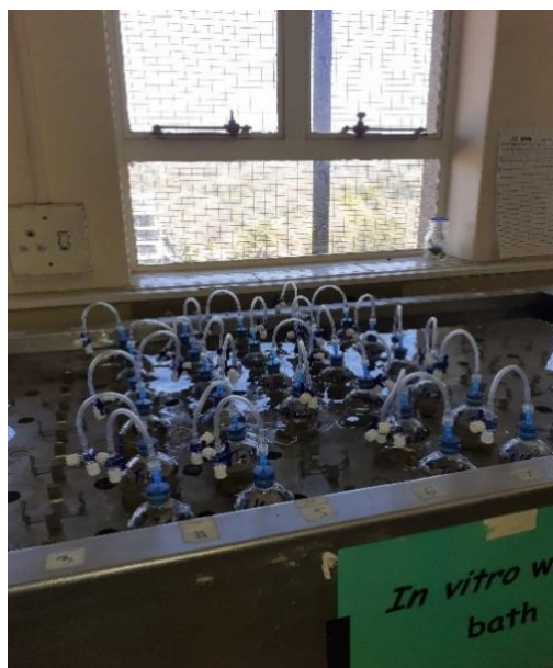
Figure 3-2 Image illustrates the 32, 100 ml bottles with rubber stoppers and a cockstopper-needle attachment in the shaking water bath maintained at 39 °C
