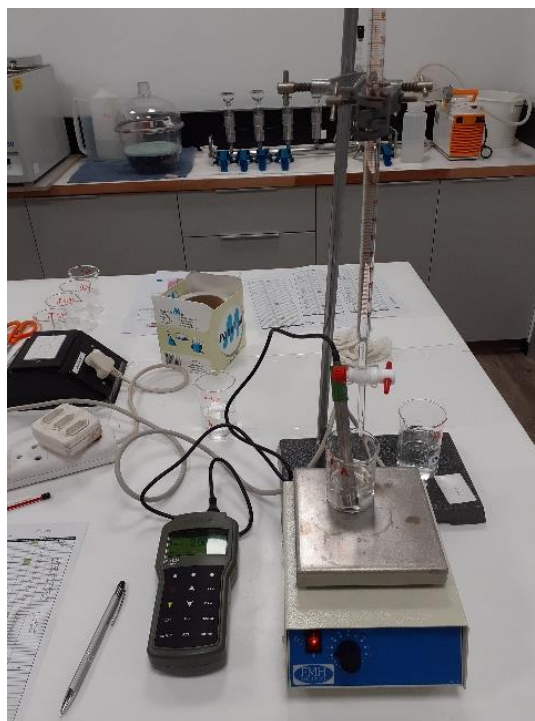
Figure 3-1 Image illustrating the arrangement of equipment for titration into aqueous-buffer solutions to determine a titration curve using a Hana portable pH meter.
