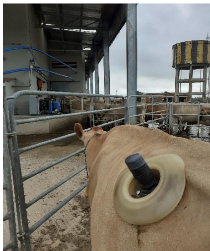
Figure 3-14 Image displays a continual pH Omni-Logger, inserted via the cannula into the rumen of an experimental animal.
