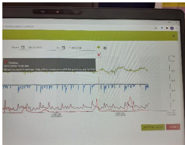
Figure 3-13 Demonstrated here are the pH-, temperature-, activity- and heat-detection-curves for a particular cow, generated every 10 minutes by the SmaXtec bolus inserted in the reticulum.
