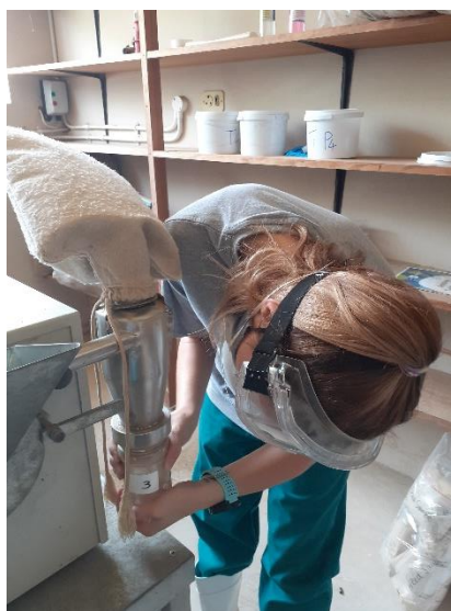
Figure 3-9 Daily faecal samples were milled through a 1 mm-sieve and pooled according to cow per treatment per period into 1 kg buckets.
