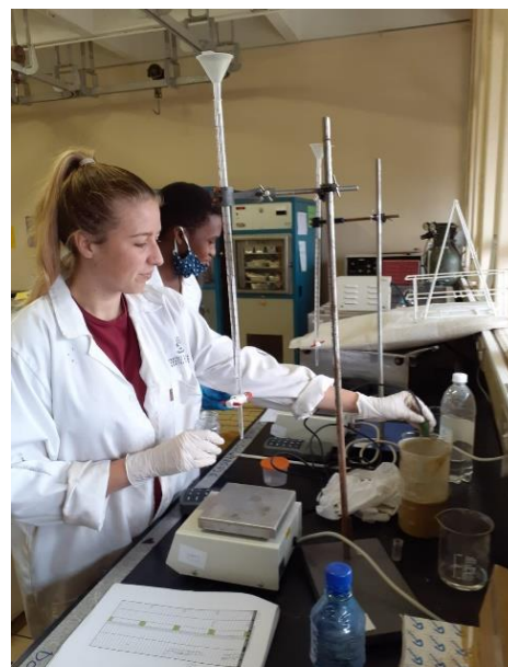
Figure 3-3 Image illustrates the setup of the titration equipment so that researchers may titrate acid and base into separate solutions simultaneously
