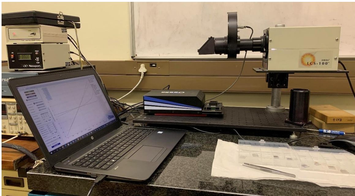
Figure 3. 10. A picture of the I-V system with the Oriel Cornerstone Newport solar simulator used in I-V measurements.
