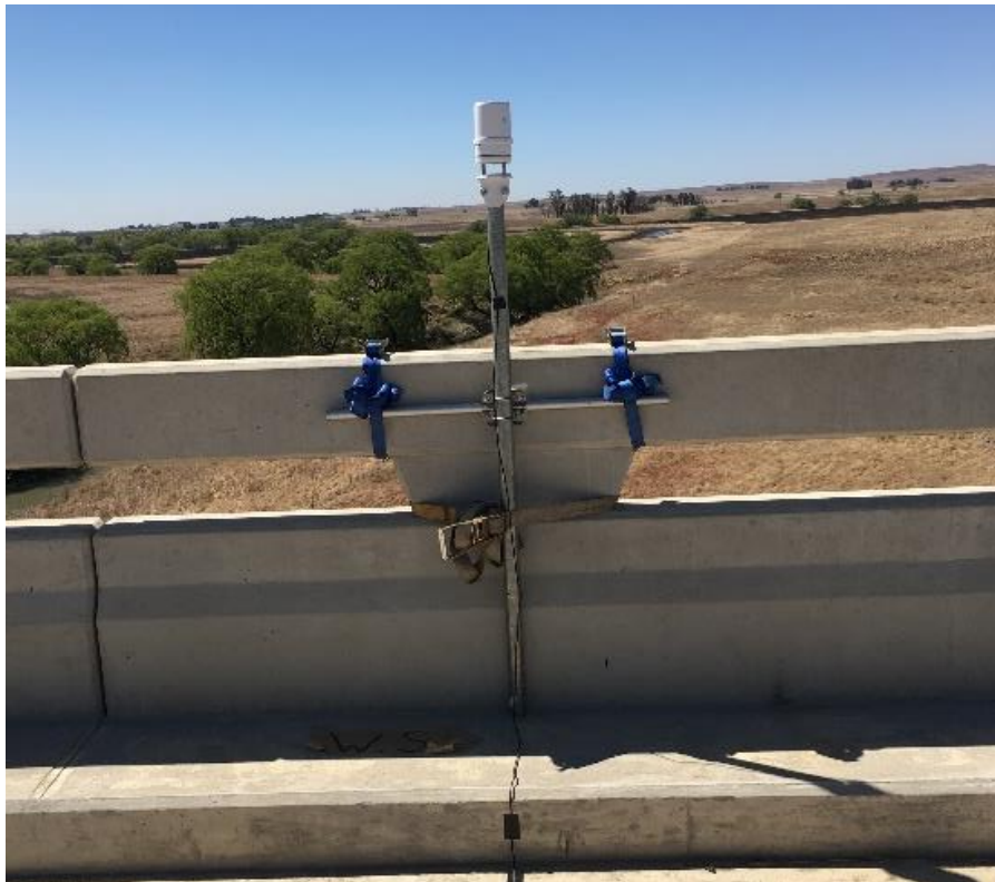
Figure 3.26: Site A - ATMOS 41 Weather Station (March 2018, September 2018)
