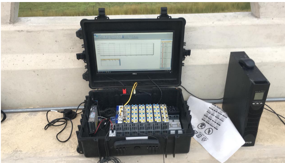
Figure 3.22: HBM QuantumX Data Logger with CATman software
