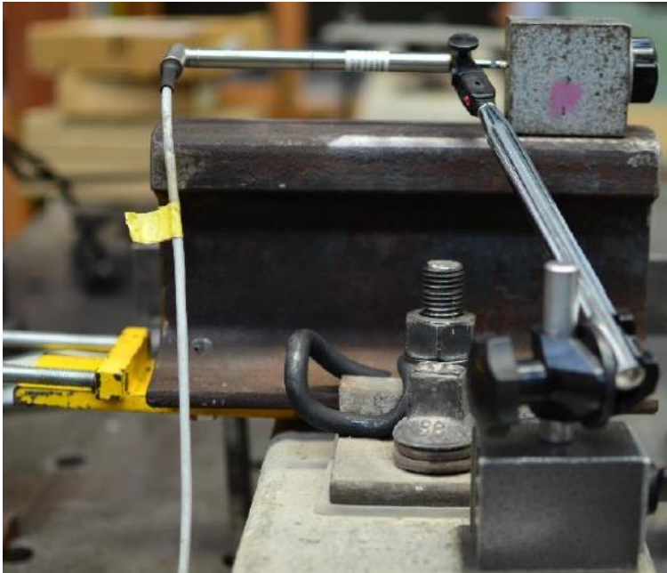
Figure 3.12: Example of longitudinal restraint test arrangement
