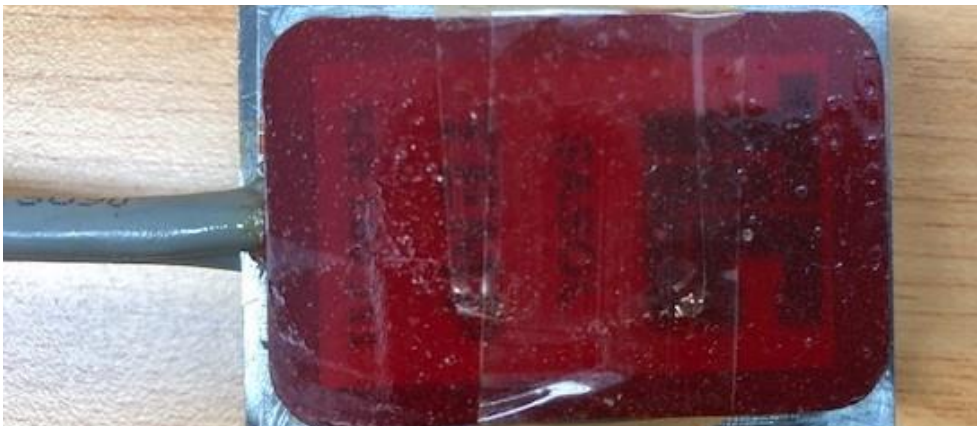
Figure 3.16: Encapsulated strain gauge supplied by TLC Engineering Solutions
