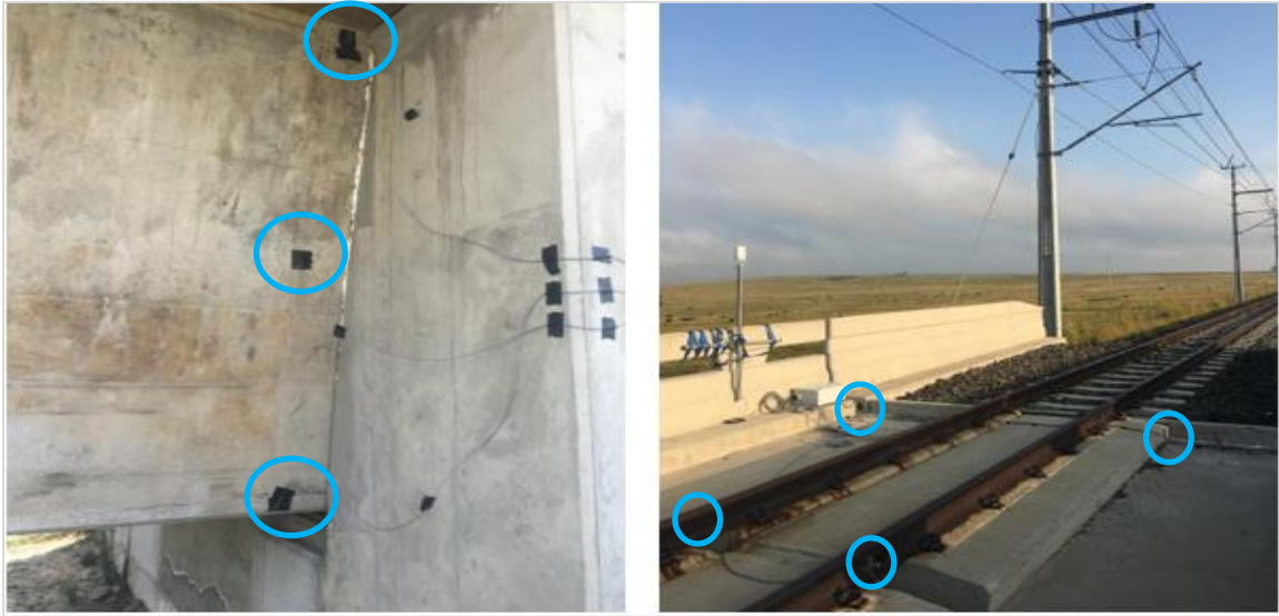
Figure 3.30: Thermistors and Weather Station at Site B (external)
