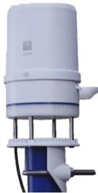
Figure 3.18: ATMOS 41 all-in-one weather station
