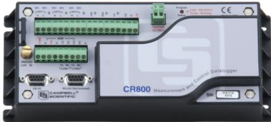
Figure 3.21: Campbell Scientific CR800 Data Logger (Campbell Scientific, 2021)
