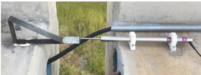
Figure 3.15: LVDT measuring bridge displacement on Majuba Rail Bridge
