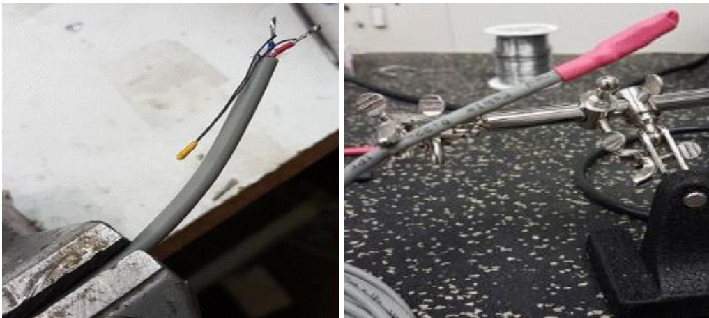
Figure 3.14: 5 k \Omega Thermistor with Heat Shrink Application
