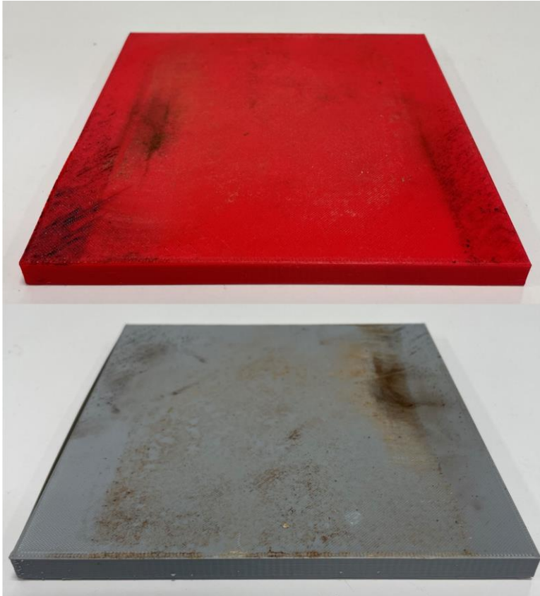
Figure 4.12: PETG (red) and PLA (grey) rail pads after 500,000 cycles
