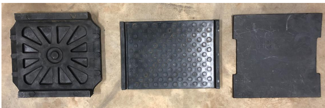
Figure 2.4: Different designs and types of rail pads: HDPE pad (left), Hytrel studded pad (middle) and a common EVA pad (right)
