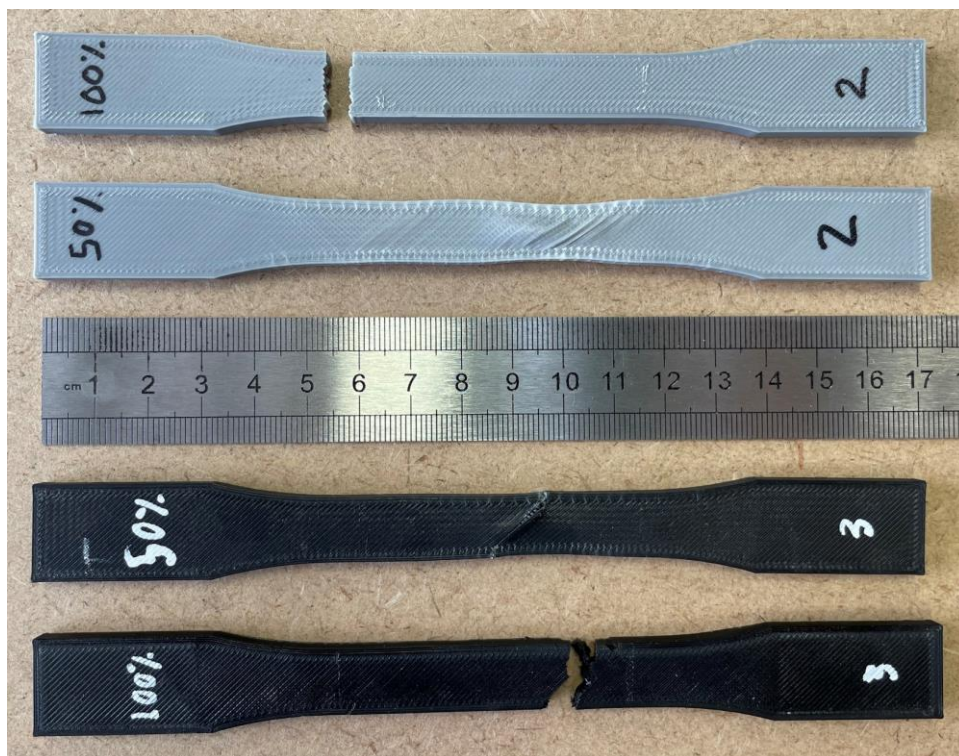
Figure 4.3: Typical brittle and ductile fracture for PETG (Black) and PLA (Grey) specimens
