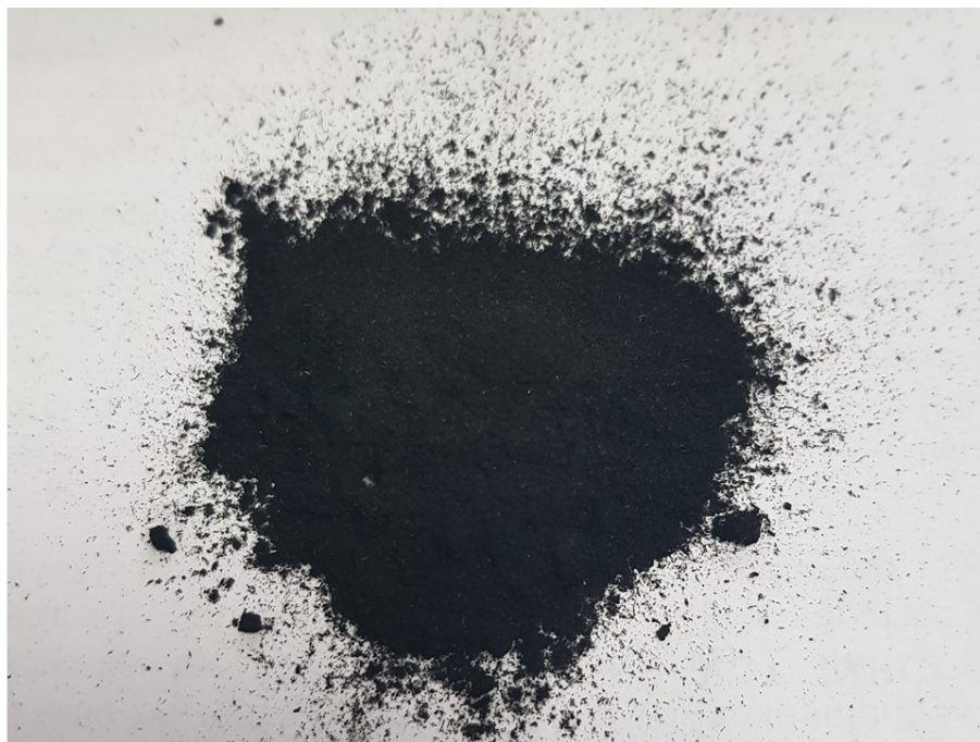
Figure 45: A sample of biochar produced from the CRIPS 2 unit
