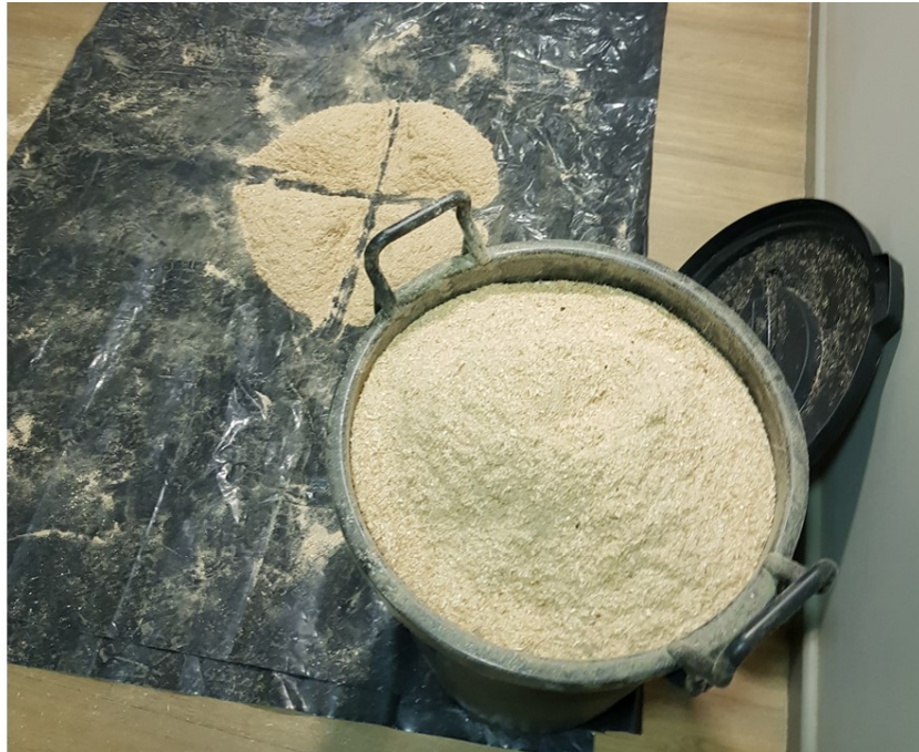
Figure 33: Example of the quartering method employed to obtain a representative biomass sample
