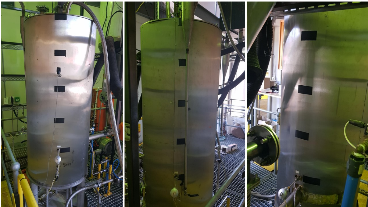
Figure 32: Photos of the temperature reading locations (black rectangles) Left to right: TR-103, TR-104, and TR-105
