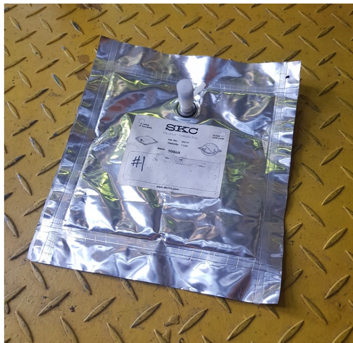
Figure 48: SKC sample bag used for NCG gas collection
