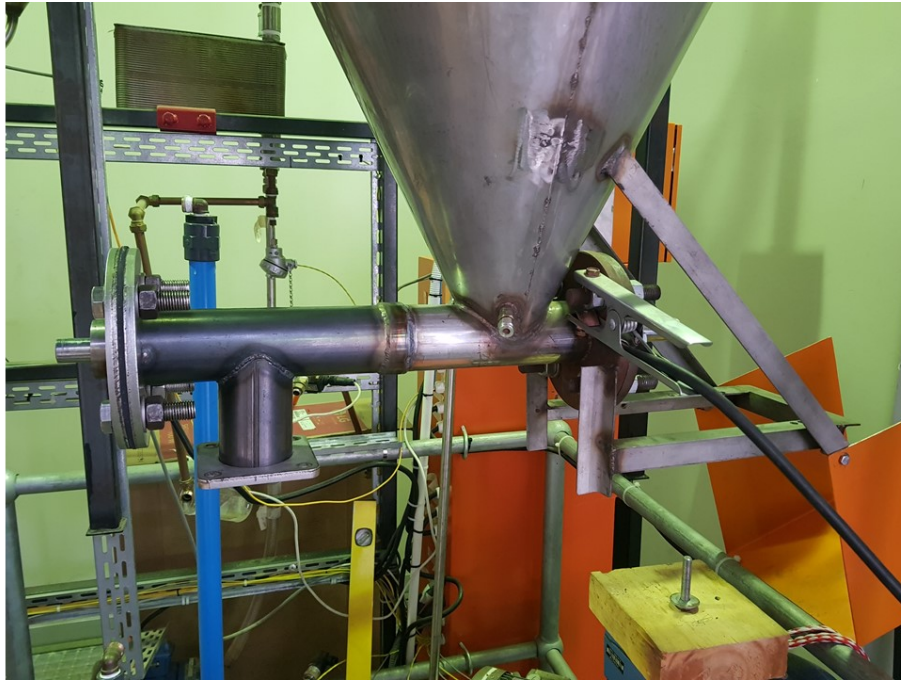
Figure 22: The final screw feeder assembly.
