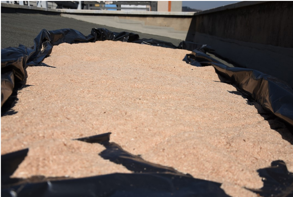
Figure 26: Drying of wood chips on the roof
