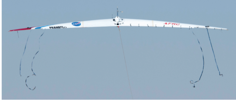
Figure 2.9: NASA's PRANDTL-D flying wing (Preliminary research aerodynamic design to lower drag) during experimental tests (Bowers et al., 2016).
