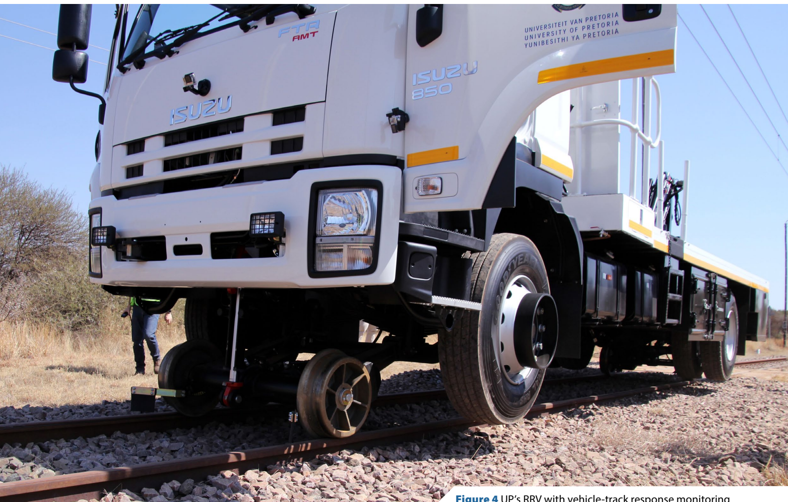
Figure 4 UP's RRV with vehicle-track response monitoring
