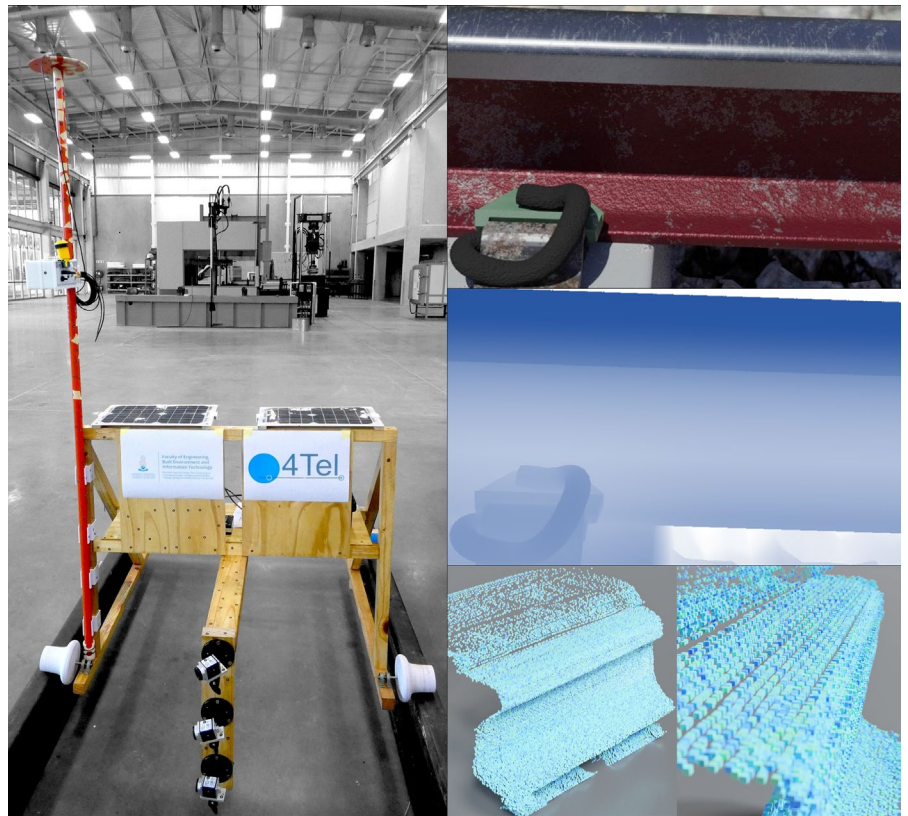
Figure 3 Camera frame (left) with GPS antenna installed and on the righthand side the synthetically rendered rail, a depth map and finally a point cloud of the railway profile
