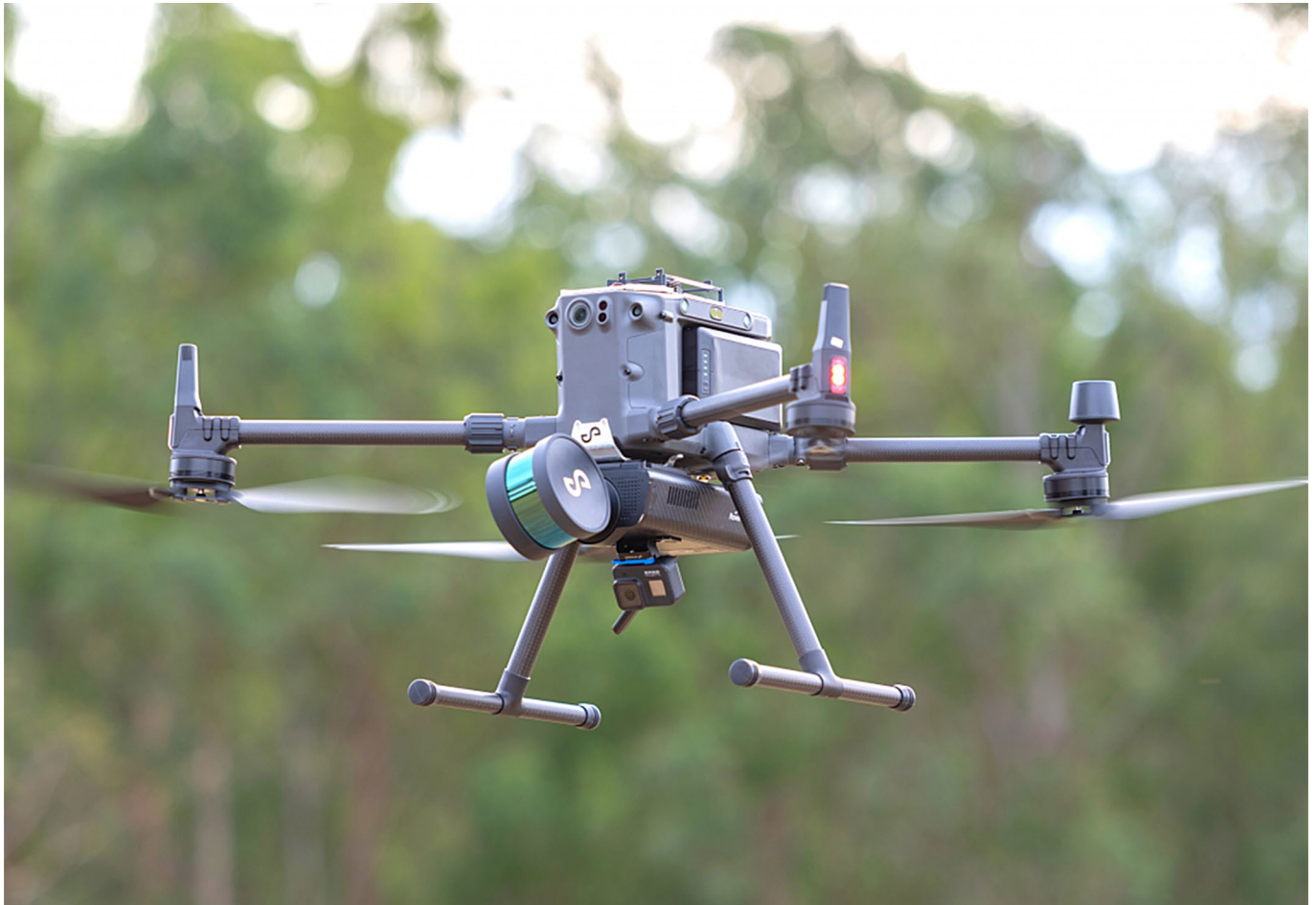
Figure 5 DJI Matrice M300 drone with Hovermap LiDAR system and GoPro colourisation
