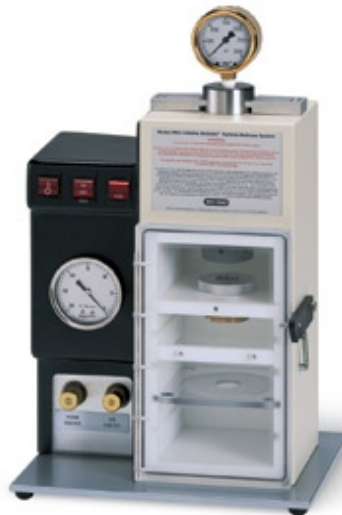
Figure 9. Bio-Rad PDS 1000/He biolistic device. Retrieved 2 March, 2014, from Bio-Rad Life Science Research: http://www.bio-rad.com/ja-jp/product/pds-1000-he-hepta-systems
