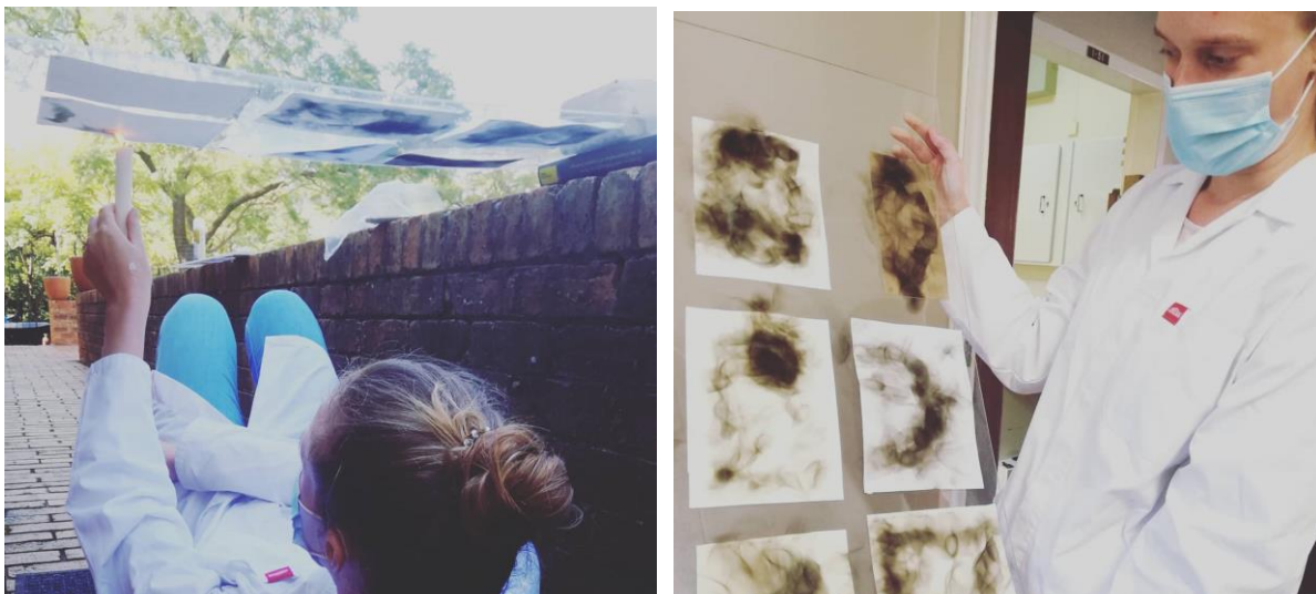
Image 1: Creating samples with candle soot (left), and some of the resulting samples (right)
