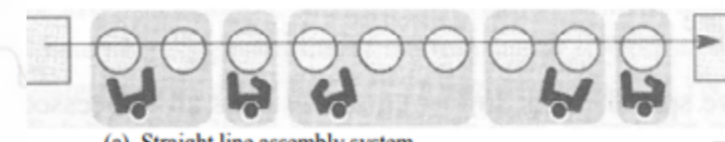
(a) Straight line assembly system
