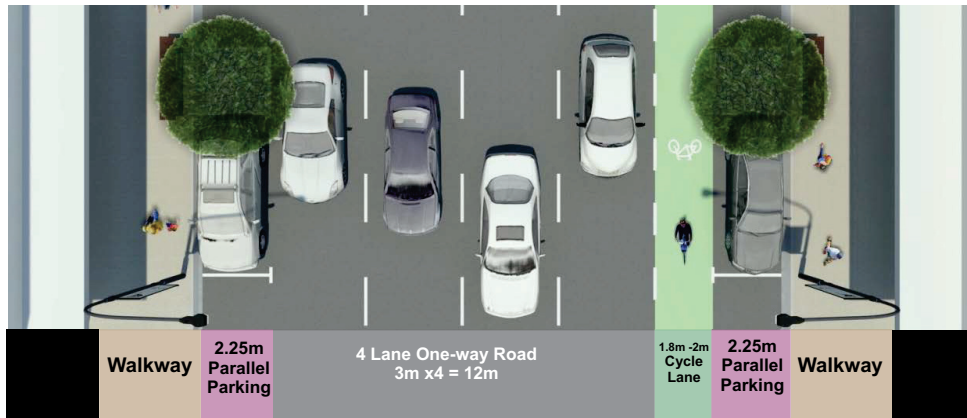
Fig 37. Image showing street plan where street design principles should be implemented (Complete Streets Design Guideline, 2019)
