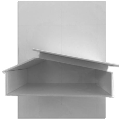
Fig. 7.5 Sectional maquette exploring South facing clerestories
