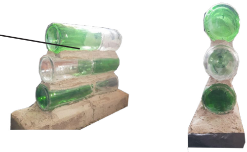
Figure 7.18: Building experiment, miniature bottle walls, mortar, brick and DIY glass bricks (Author 2021)
