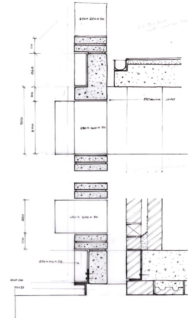
Fig. 126: Exploration of precast concrete screen (Author 2021)
