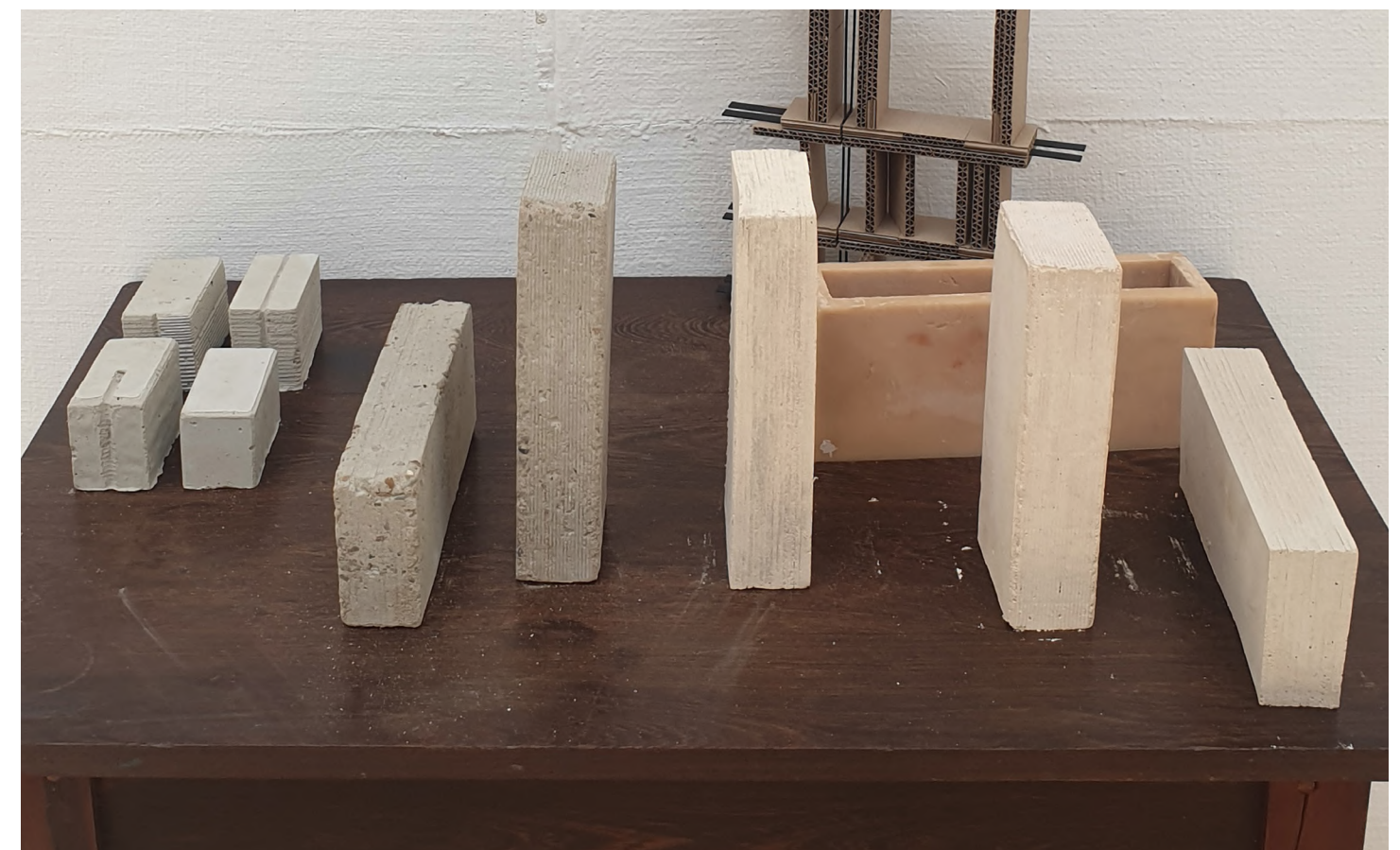
Fig. 128: Full scale precast concrete brick castings (Author 2021)
