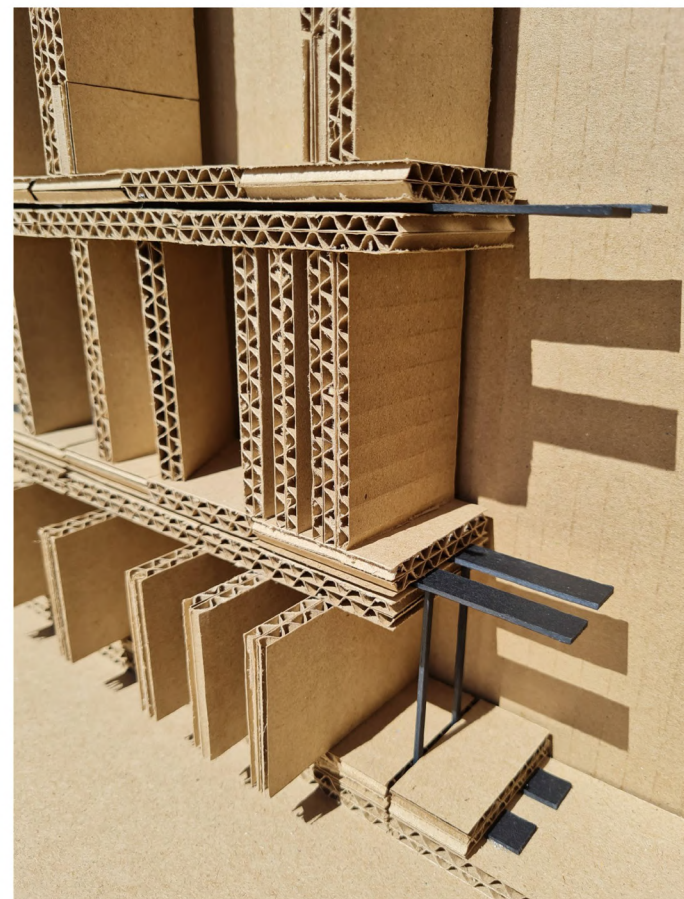
Fig. 127: 1:5 model of the screen's structural system. An iteration using steel reinforcement. (Author 2021)
