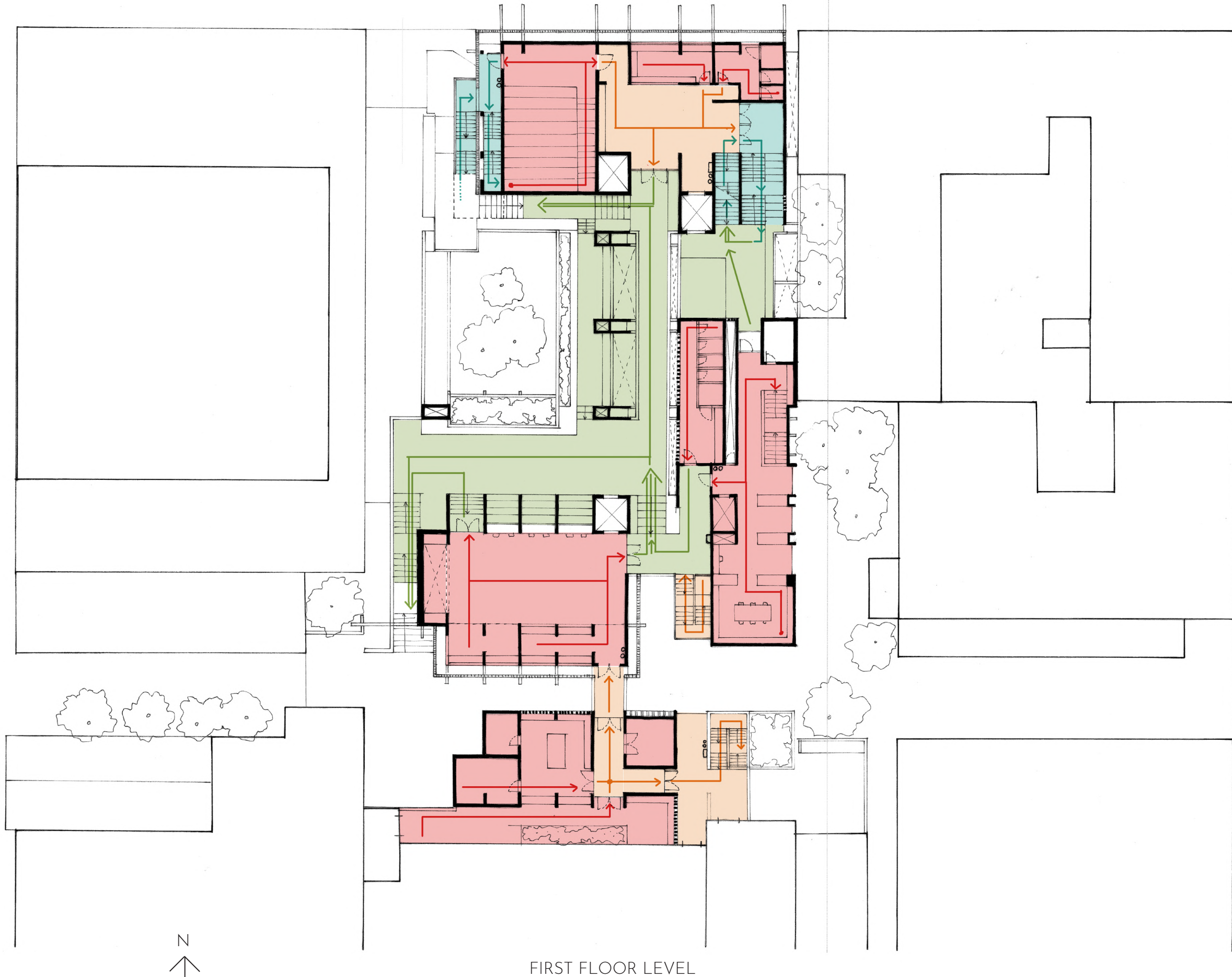
Fig. 160: Plan of first floor level indicating escape routes (Author 2021)
