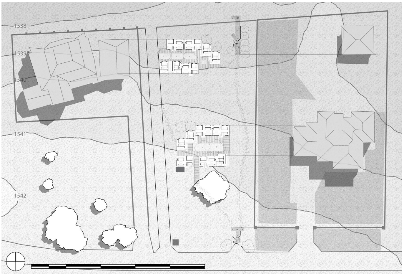
Figure 92: Site plan of the arrival pavilion depicting thresholds and accommodation units. A service delivery road on the western side links to existing dirt roads on the site. As a threshold between the suburbs and ruin landscape, the various components are placed in relation to the geometry of the surroundings as a means of connecting the two entities (Author, 2021).
