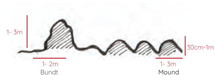
Fig 99: Sectional diagrams through bunds and yam mounds at the buffer (van Staden 2021).
