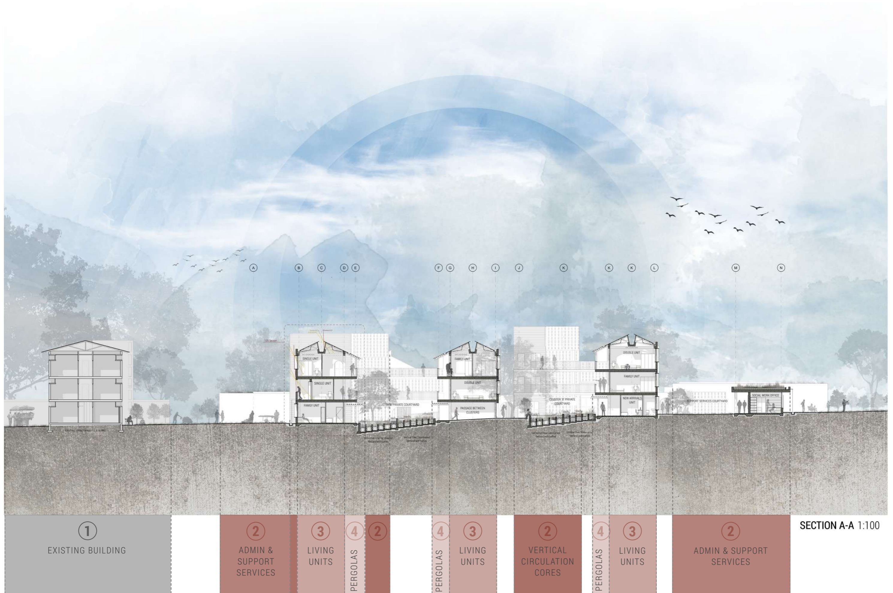
Final Section A-A at scale 1:100 on A0 landscape, indicating various spaces according to their levels of permanence (Author 2021).
