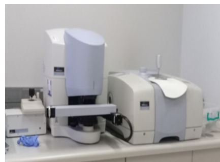
Figure 2: FTIR spectrometer (Perkin Elmer Spectrum 100) with an ATR
